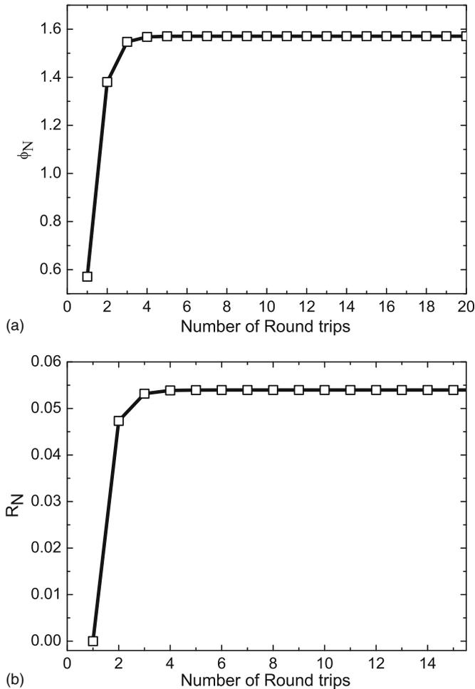
**Figure 3.** (a)  $\phi_N$  vs. number of round trips and (b)  $R_N$  vs. number of round trips for  $\omega = 2\pi$ .
