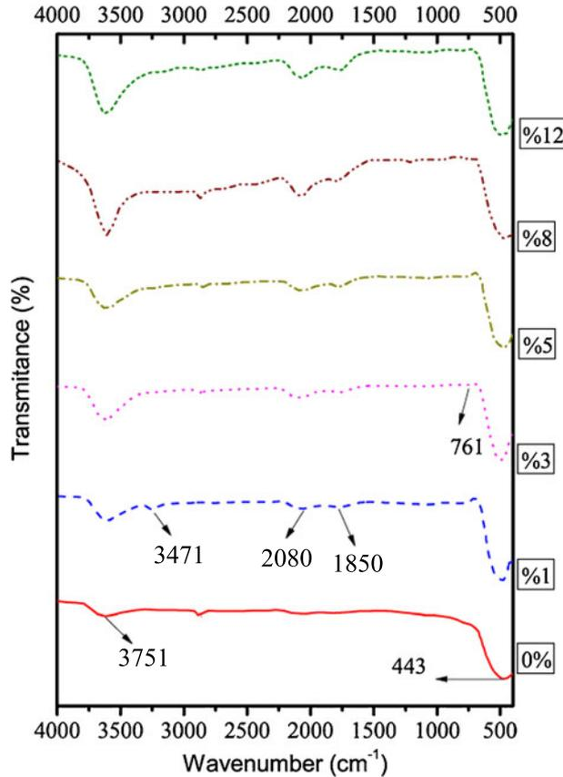
**Figure 3.** FTIR spectra of Mn-doped ZnO at 0, 1, 3, 5, 8, and 12 wt% Mn doping concentrations.
