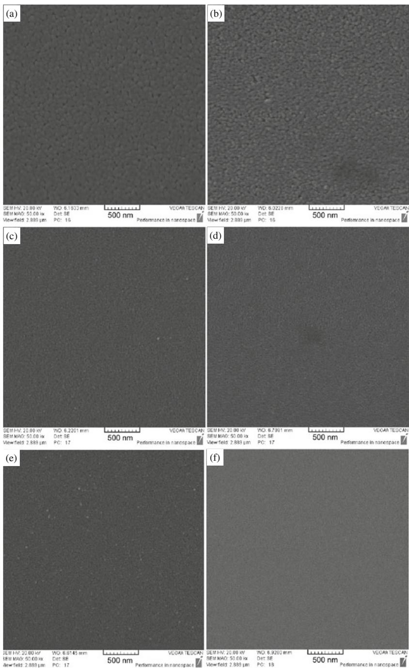
**Figure 2.** SEM micrographs of nanostructured ZnO:Mn thin films at various Mn concentrations, (a) undoped, (b) 1 wt%, (c) 3 wt%, (d) 5 wt%, (e) 8 wt%, and (f) 12 wt%.
