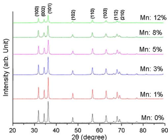
**Figure 1.** XRD patterns of ZnO:Mn thin films at 0, 1, 3, 5, 8 and 12 wt% Mn concentrations.
