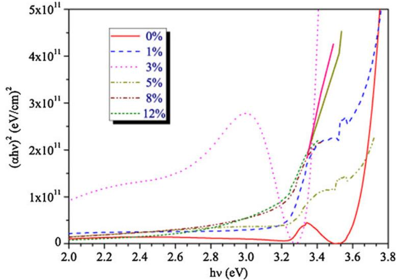
**Figure 5.** The plots of  $(\alpha hv)^2$  vs. photon energy of nanostructured ZnO:Mn thin films.
