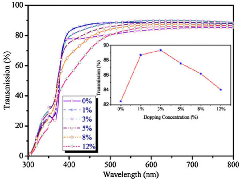
Figure 4. The transmission spectra of the Mn-doped ZnO thin films vs. wavelength.
