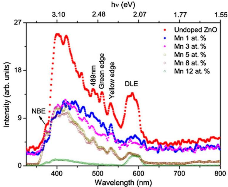
**Figure 6.** Photoluminescence (PL) spectra of ZnO:Mn thin films with various Mn concentrations.
