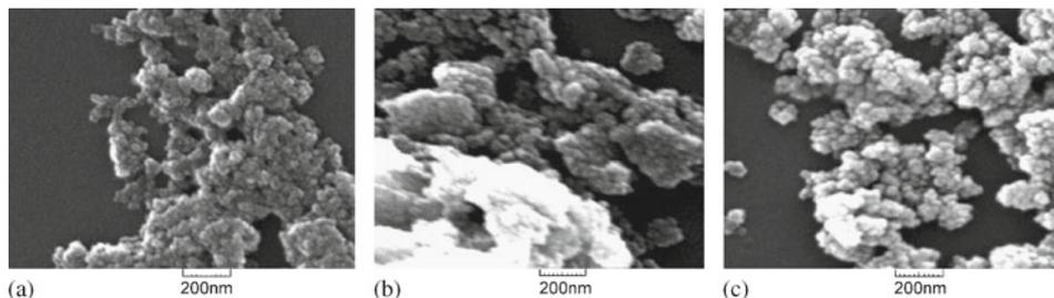
**Figure 8.** SEM images of ZnO annealed at different temperatures: (a) 100°C, (b) 200°C and (c) 400°C.
