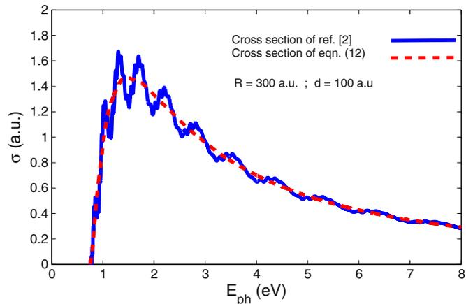
**Figure 5.** A comparison of the photodetachment cross-section of eq. (12) and that of ref. [2] is shown.
