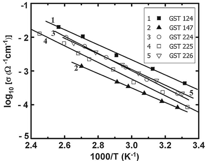
**Figure 3.** Conductivity as a function of inverse temperature of amorphous GST films. Here GST 124 corresponds to  $\text{Ge}_1\text{Sb}_2\text{Te}_4$  and so on. The activation energies ( $E_\sigma^*$ ) are given in table 1 (after [16]).
