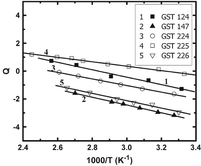
**Figure 5.** Variation of  $Q$  as a function of inverse temperature of amorphous GST samples.  $Q$  is defined in eq. (7), so that it is independent of the position of Fermi level (after [16]).
