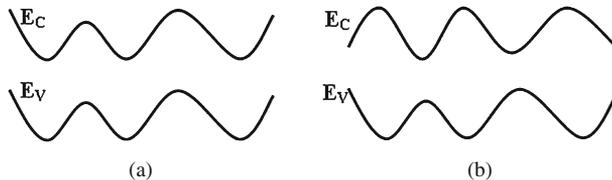
**Figure 6.** Band edge fluctuations in amorphous semiconductors (a) symmetric (b) antisymmetric.
