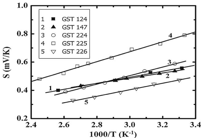
**Figure 4.** Variation of thermopower of GST alloys as a function of inverse temperature. The slopes ( $E_S^*$ ) are listed in table 1 (after [16]).
