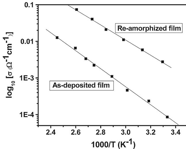
**Figure 10.** Conductivity  $\sigma(T)$  data of an ‘as-deposited’ amorphous GST 225 film compared with the re-amorphized GST 225 film.
