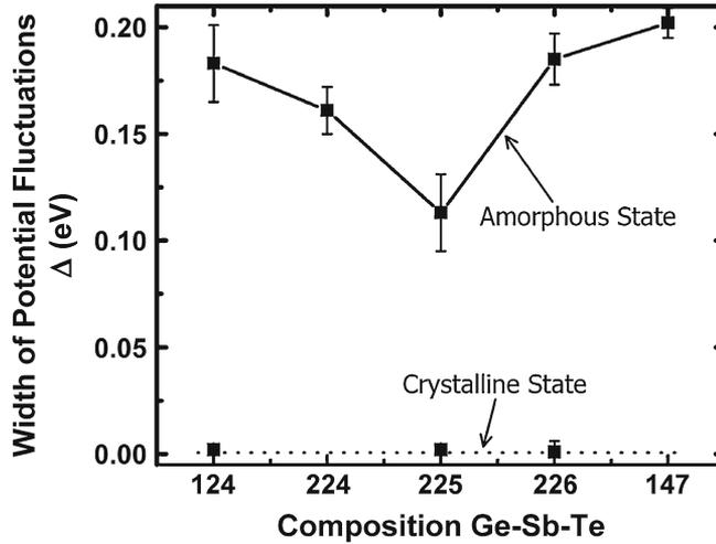
**Figure 9.** Widths of potential fluctuations ( $\Delta$ ) calculated and tabulated (table 1) for GST samples in amorphous and crystalline phases. The GST 225 film shows the smallest potential fluctuations compared to the other compositions. Note that  $\Delta$  in crystalline phase is zero [17].
