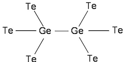
**Figure 2.**  $\text{Ge}_2\text{Te}_3$  configuration, as might be present in  $\text{Ge}_2\text{Sb}_2\text{Te}_5$  (after ref. [19]).
