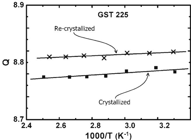
**Figure 8.**  $Q$  as a function of inverse temperature for crystallized and re-crystallized GST 225. Please note the reproducibility of the slope.
