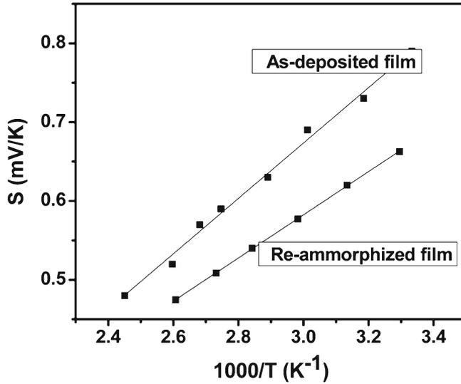
**Figure 11.** Comparison of thermopower  $S(T)$  of a GST 225 film in the ‘as-deposited’ and re-amorphized states.
