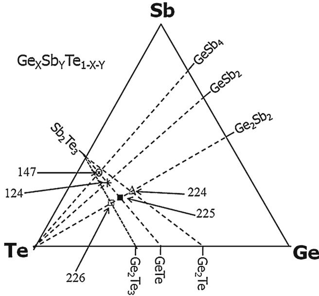
**Figure 1.** Ternary phase diagram for Ge–Sb–Te compounds, showing locations of compounds considered in this article, and the various tie-lines.
