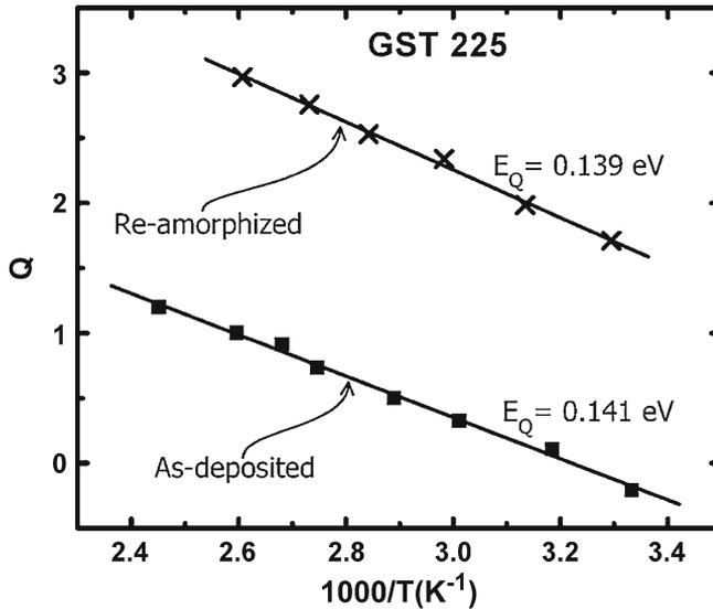
**Figure 12.** Comparison of  $Q$  of an as-deposited GST 225 film and re-amorphized film as a function of inverse temperature  $T$ . Please note that although  $\sigma(T)$  and  $S(T)$  change after re-amorphization (figures 10 and 11),  $Q(T)$  remains unchanged [17].
