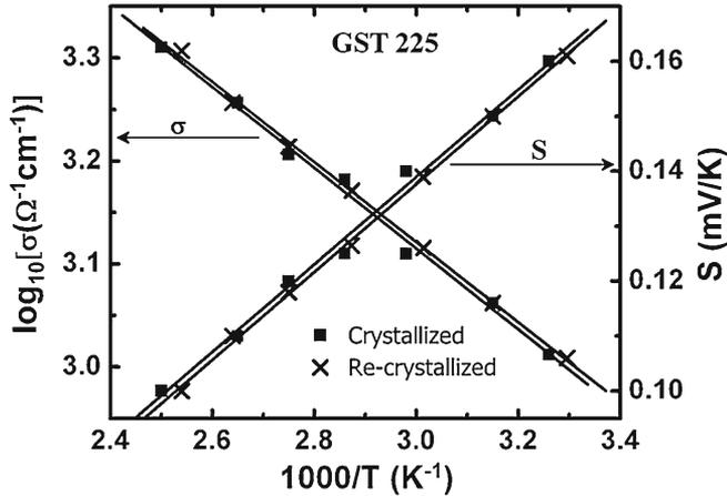
**Figure 7.** Log conductivity ( $\sigma$ ) and thermopower ( $S$ ) of crystallized and re-crystallized GST 225 as a function of inverse temperature (please note the two ordinate scales for  $\sigma$  and  $S$ ). The data are essentially unchanged after re-crystallization [17].
