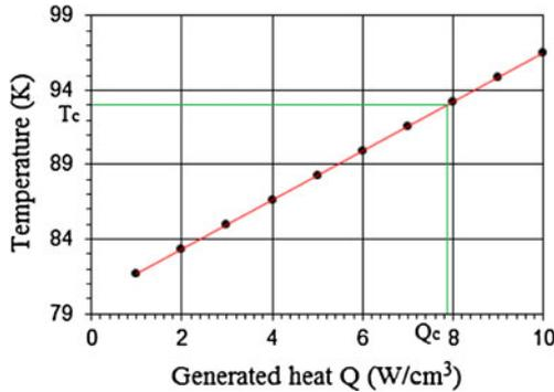
**Figure 3.** Temperature along the length of YBCO tape for different heat generation for a given time period of  $t = 2.0$  s, excluding both the edges.
