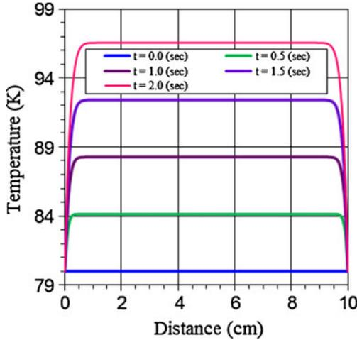
**Figure 2.** Temperature of YBCO tape with respect to the position coordinate for different times.
