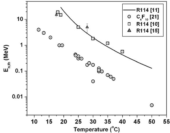
**Figure 3.** Variation of threshold neutron energy ( $E_{n,th}$ ) with temperature for  $C_4F_{10}$  and R114.
