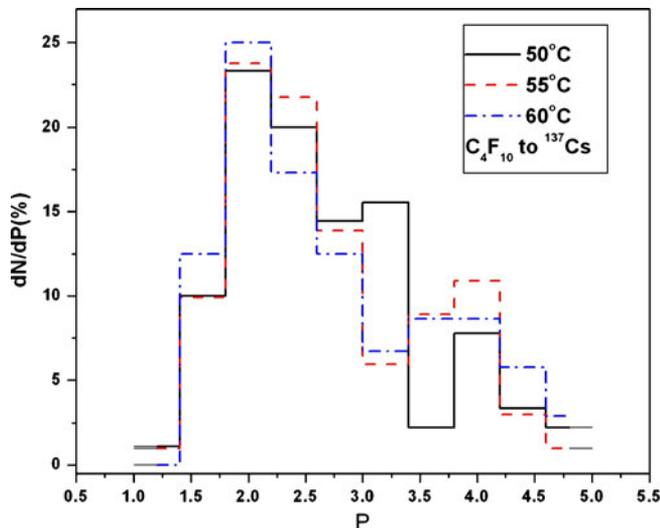
**Figure 2.** Observed differential power distribution of pulses of  $C_4F_{10}$  detector in the presence of  $^{137}Cs$   $\gamma$ -source.
