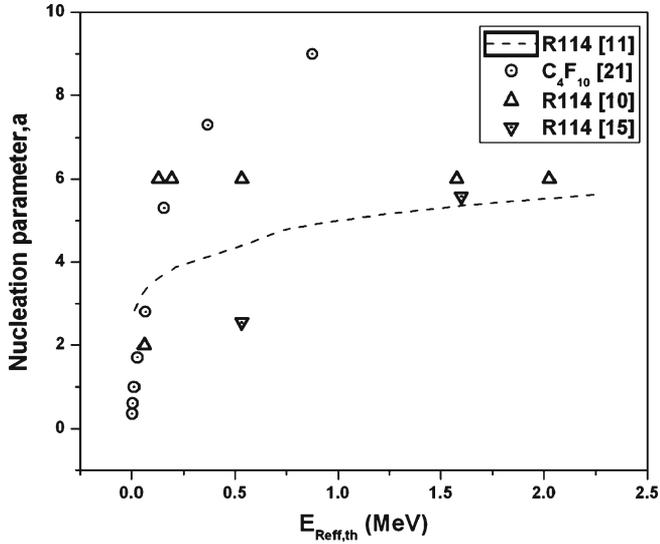
**Figure 9.** Nucleation parameter  $a$  as a function of effective recoil nucleus threshold energy  $E_{\text{Reff,th}}$ .
