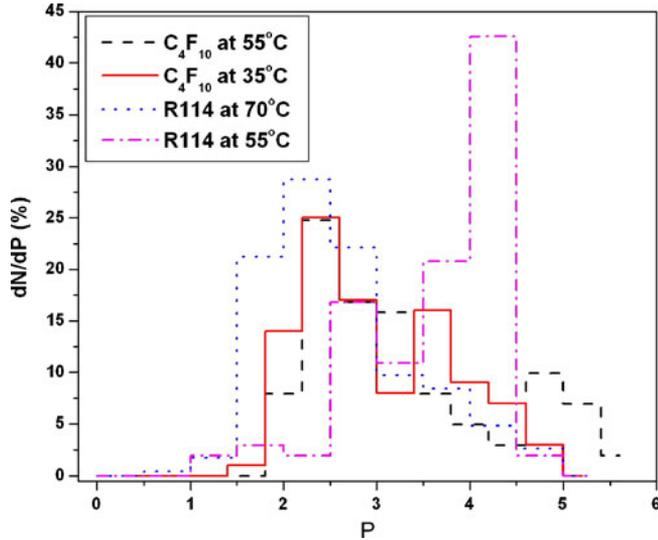
**Figure 5.** Observed differential power distributions at different temperatures for  $C_4F_{10}$  and R114 in the presence of  $^{252}Cf$  fission neutron source.
