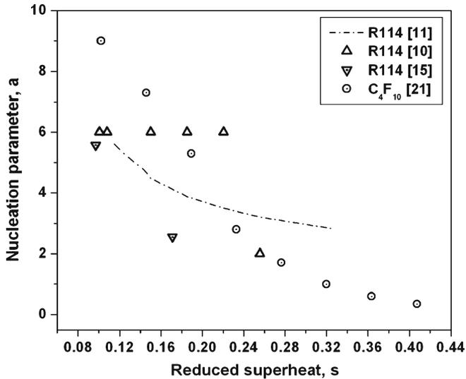
**Figure 10.** Nucleation parameter  $a$  as a function of reduced superheat  $s$ .
