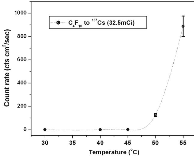
**Figure 1.** Observed response of  $C_4F_{10}$  detector as a function of temperature in the presence of  $^{137}Cs$   $\gamma$ -source.
