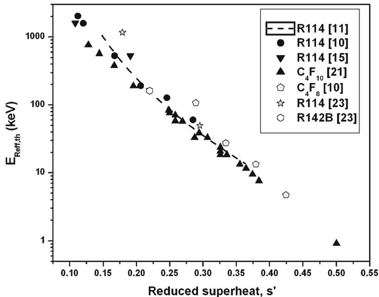
**Figure 8.** Variation of effective recoil nucleus threshold energy  $E_{\text{Reff,th}}$  as a function of reduced superheat  $s'$ .
