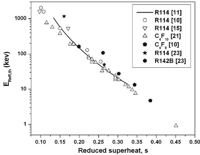
**Figure 7.** Variation of effective recoil nucleus threshold energy  $E_{\text{Reff,th}}$  as a function of reduced superheat  $s$ .
