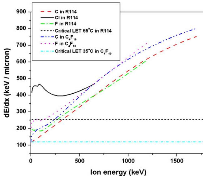
**Figure 4.** Variation of  $dE/dx$  for C, Cl, F in R114 and for C, F in  $C_4F_{10}$ .
