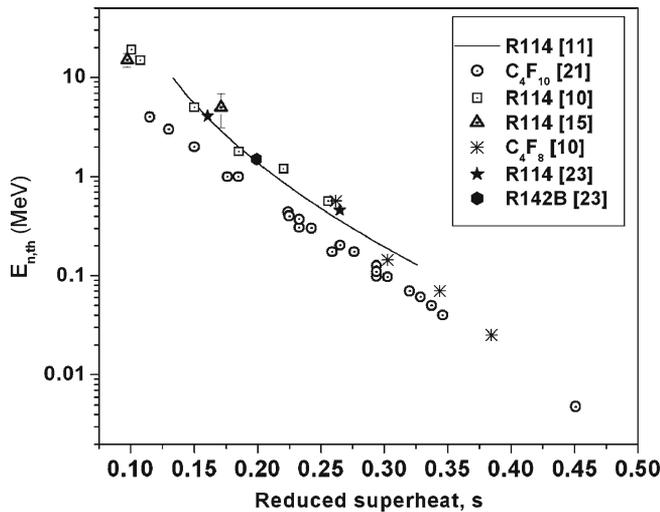
**Figure 6.** Variation of threshold neutron energy  $E_{n,th}$  as a function of reduced superheat  $s$  for different liquids.
