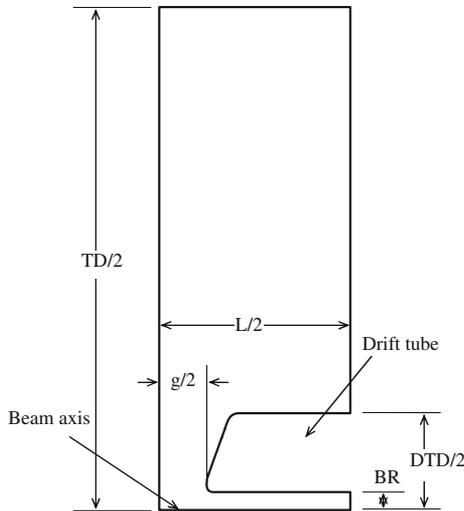
**Figure 2.** 1/4th unit cell drift tube geometry.
