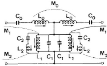
**Figure 8.** Equivalent circuit of a post-coupled structure.
