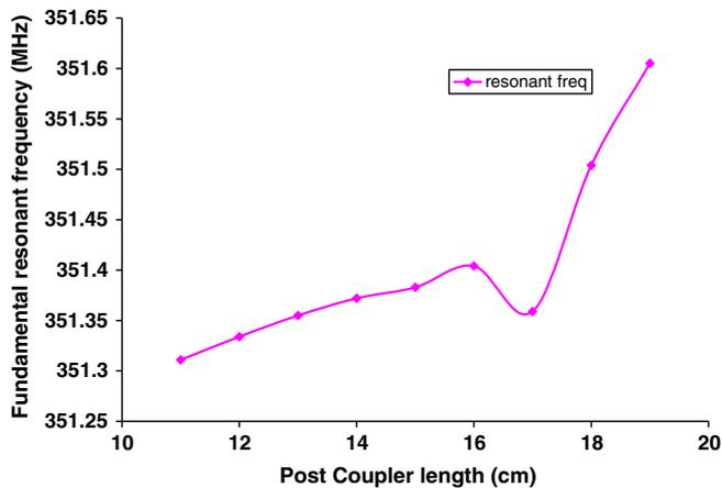
Figure 13. Resonant frequency vs. post-coupler length for a post-coupler radius of 1.3 cm.
