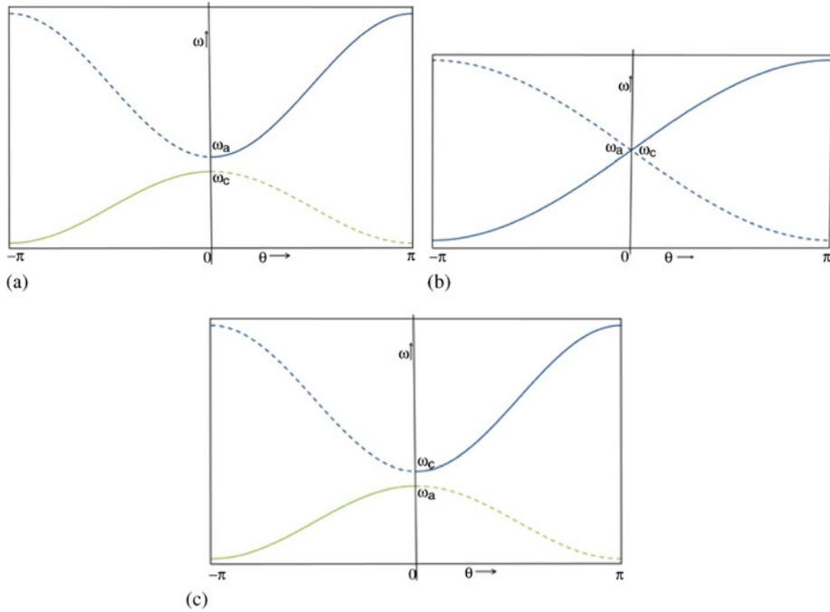
**Figure 7.** Dispersion curve of a structure with resonant coupling. (a) Undercompensated case, (b) compensated case and (c) overcompensated case.
