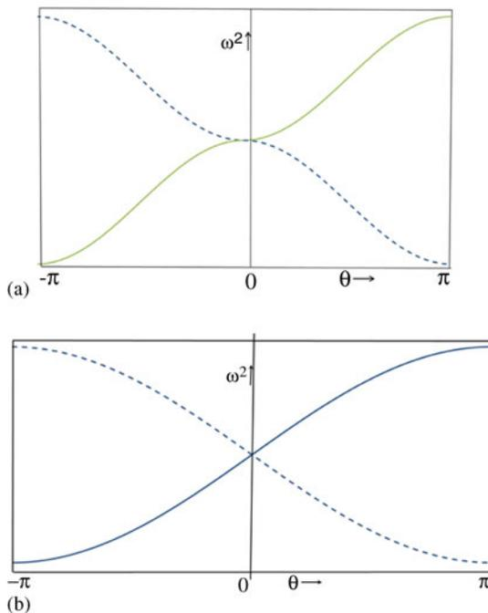
**Figure 6.** Confluence of two pass-bands (a) without coupling and (b) with coupling between the two merging pass-bands, i.e. the stabilized case.
