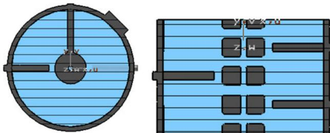
**Figure 9.** Drift tube tank with drift tube and post-coupler simulated using CST MWS.
