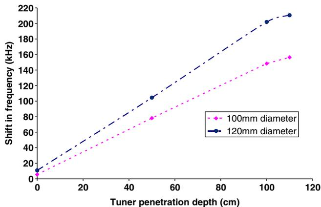
Figure 4. Tuner penetration depth vs. shift in resonant frequency.
