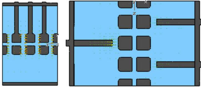
**Figure 10.** Field configuration for the fundamental mode ( $TM_{010}$ ) and the lowest order post-coupled mode (TE) using CST MWS.
