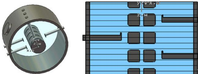
**Figure 11.** Post-couplers with tab generated using CST MWS.
