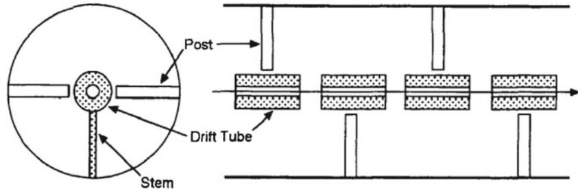
**Figure 5.** Drift tube Linac with post-couplers for field stabilization.
