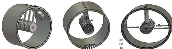
Figure 3. CST MWS plots showing tuner, vacuum port and post-couplers.
