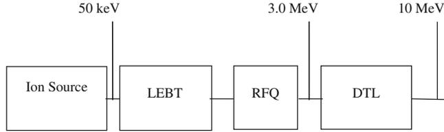
**Figure 1.** Lay-out of the Linac front end.
