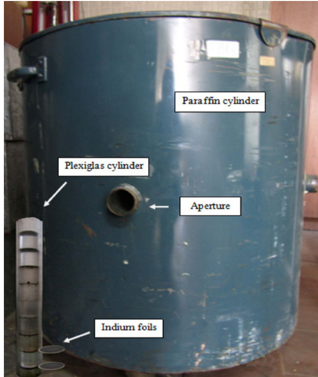
Figure 2. A view of paraffin phantom, Plexiglas cylinder, indium foils and aperture. Neutron source is 18 cm above the aperture.
