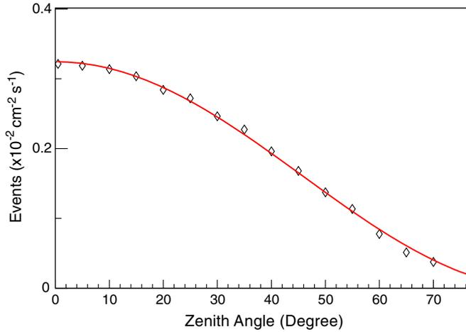
**Figure 4.** Zenith angle dependence of cosmic muons at sea level using Geant4 simulation package.
