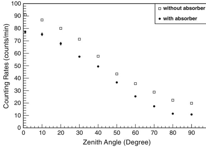
**Figure 1.** Angular distributions of cosmic muons at sea level measured using a Berkeley Lab cosmic ray detector (■) with and (□) without absorber material between the scintillation paddles.
