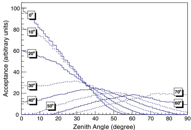
Figure 2. Acceptance of the Berkeley Lab cosmic ray detector at each measurement orientation.
