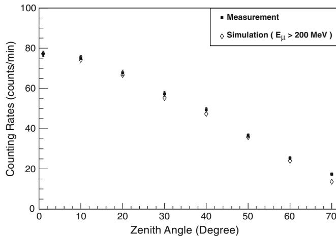
**Figure 3.** Zenith angle dependence measurements at sea level using a Berkeley Lab cosmic ray detector with (■) absorber between the scintillation plates and (◇) normalized simulation counts. Normalization was made at  $\theta = 0^\circ$ .
