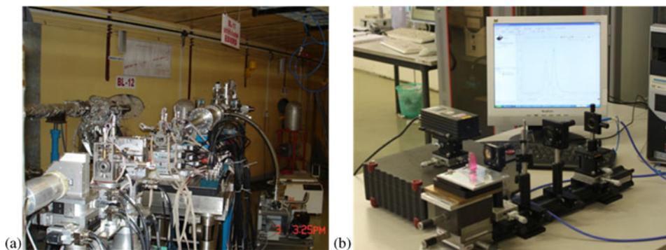
**Figure 6.** (a) EDXRD beamline, (b) off-line ruby pressure measurement set-up.
