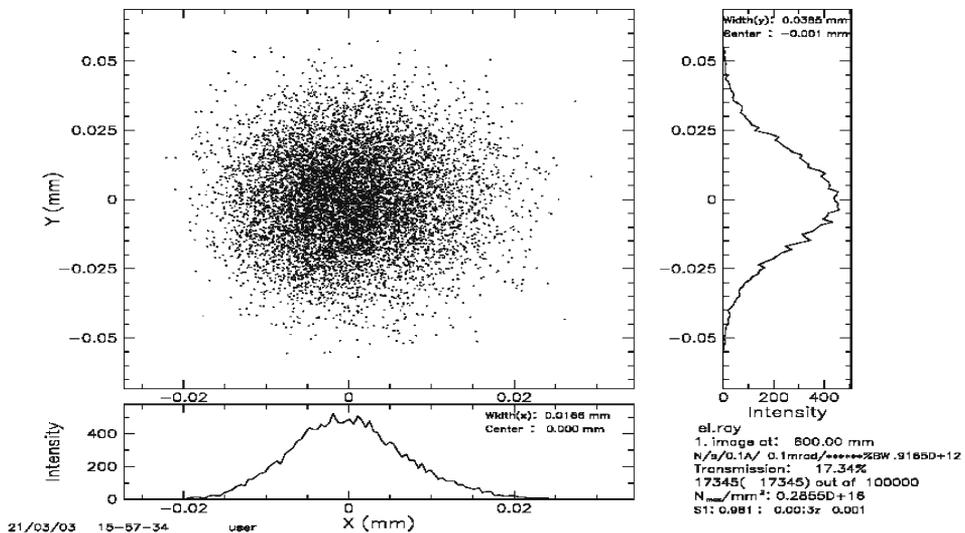
Figure 2. Ray tracing simulation of focal spot size using a KB mirror system.
