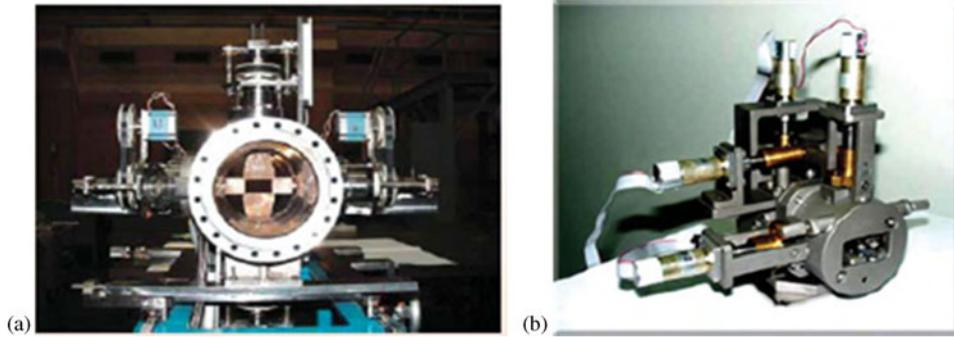
Figure 1. (a) Primary slit system, (b) precision slit system.
