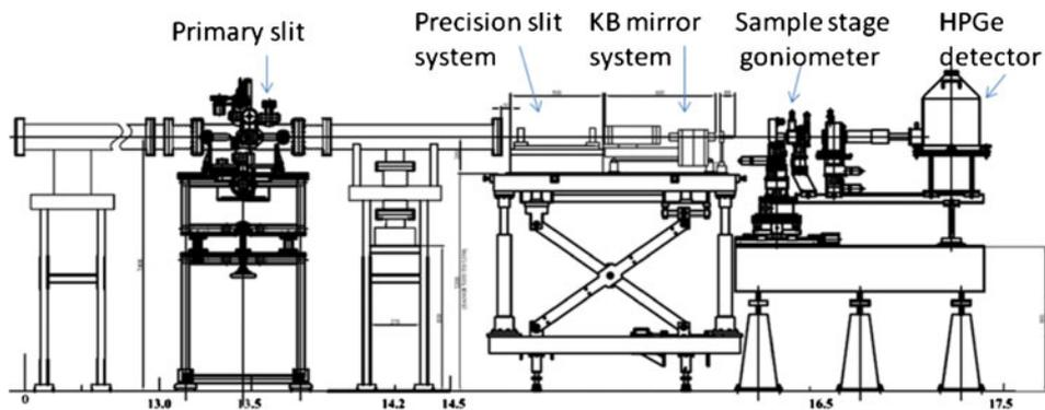
Figure 5. Mechanical lay-out of EDXRD beamline.
