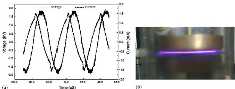
**Figure 2.** (a) Voltage and current waveforms of the APGD produced with a power supply operated at 26.5 kHz, gap spacing = 0.5 mm, thickness of the dielectric (glass) = 2 mm. (b) Photograph of the discharge.
