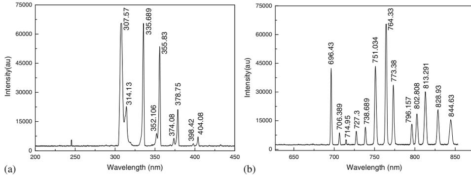
**Figure 6.** Ar lines obtained from the APGD in the range of 200–450 nm (a) and 650–850 nm (b).
