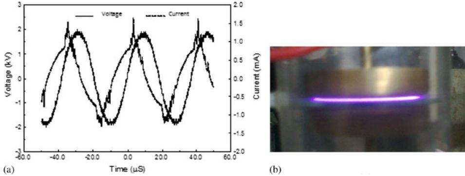
**Figure 3.** (a) Voltage and current waveforms of the APGD produced with a power supply operated at 26.5 kHz, gap spacing = 1 mm, thickness of the dielectric (glass) = 2 mm. (b) Photograph of the discharge.
