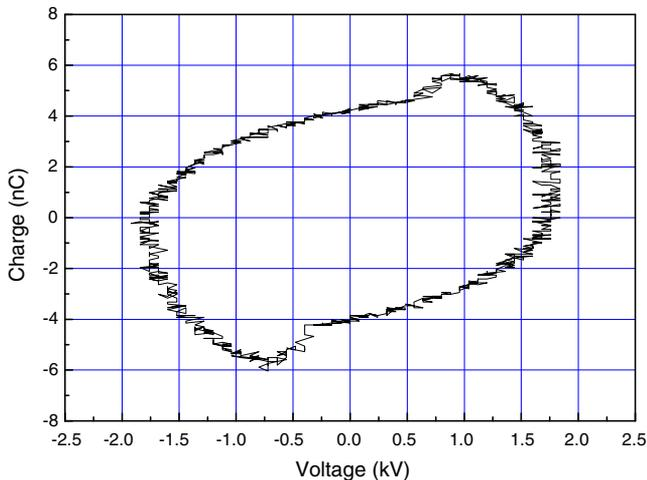
**Figure 9.** Lissajous figure of APGD with an electrode spacing of 0.5 mm.
