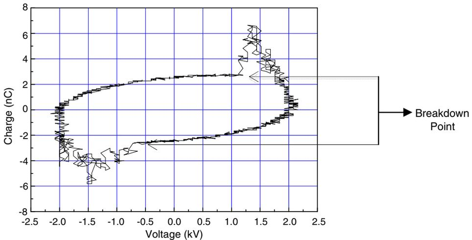
**Figure 11.** Lissajous figure of APGD with an electrode spacing of 2 mm. Arrows show the points when breakdown occur.
