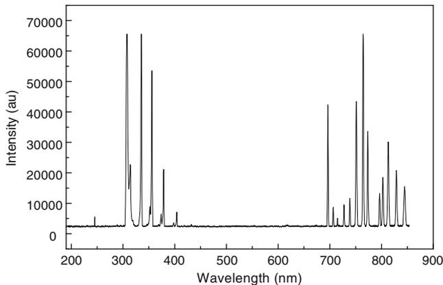
**Figure 5.** Optical emission lines of atmospheric pressure APGD produced in Ar.
