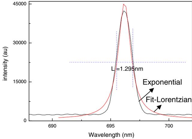
**Figure 8.** Recorded line profile for  $\lambda_{n1} = 696.54$  nm and its Lorentzian fit.
