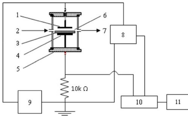
**Figure 1.** Schematic diagram of the experimental set-up. 1 – Electrode, 2 – gas inlet, 3 – dielectric, 4 – grounded electrode, 5 – bottom flange, 6 – discharge gap, 7 – gas outlet, 8 – HV probe, 9 – HV power supply, 10 – digital oscilloscope, 11 – PC.
