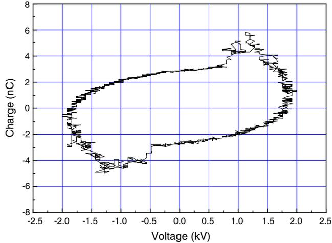
**Figure 10.** Lissajous figure of APGD with an electrode spacing of 1 mm.
