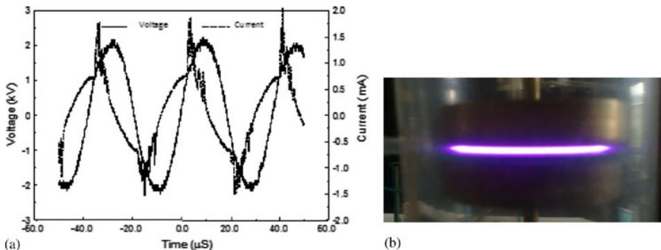
**Figure 4.** (a) Voltage and current waveforms of the APGD produced with power supply operated at 26.5 kHz, gap spacing = 2 mm, thickness of the dielectric (glass) = 2 mm. (b) Photograph of the discharge.
