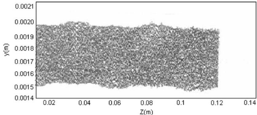
**Figure 3.** One and a half-dimensional PIC simulation of wiggler transport using TUBE.
