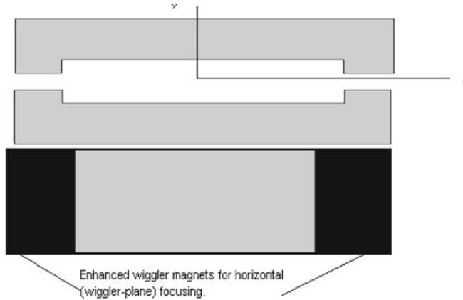
**Figure 1.** Shape of the wiggler magnets for horizontal (wiggler-plane) focussing.
