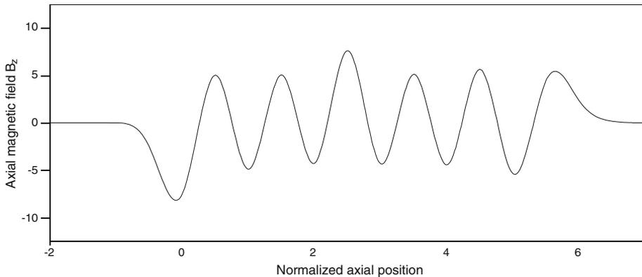
**Figure 2.** Numerically calculated axial magnetic field component  $B_z$  in kG of the notched wiggler magnet array as displayed in figure 1 for  $x = 0$  and  $y = 0$ .
