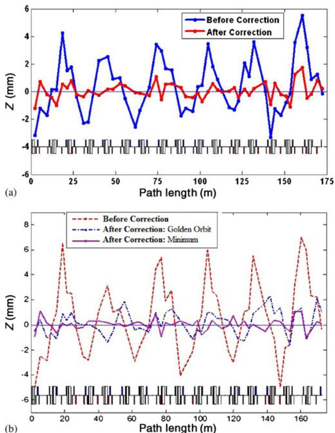
**Figure 5.** (a) Vertical COD before and after correction at 550 MeV. (b) Vertical COD before and after correction at 2 GeV. Dotted line shows the orbit before correction, dash-dotted line shows after correction for the beamline users (golden orbit) and solid line shows the minimum possible corrected orbit.
