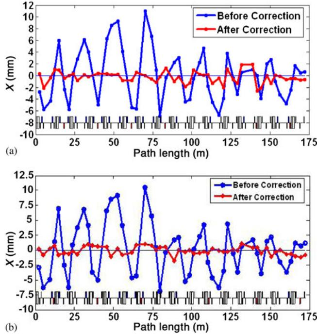
**Figure 4.** (a) Horizontal COD before and after correction at 550 MeV injection energy and (b) at 2 GeV.
