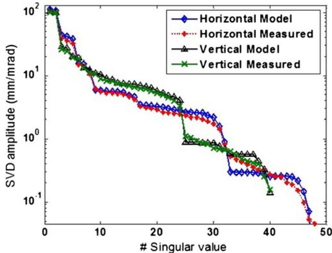
**Figure 3.** Singular value decomposition of the model and measured response matrices in the horizontal and vertical planes at 2 GeV.
