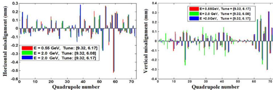
**Figure 2.** Effective misalignments of the quadrupoles in horizontal and vertical planes calculated by fitting the measured COD at 550 MeV injection energy and at final energy 2 GeV for various betatron tunes.
