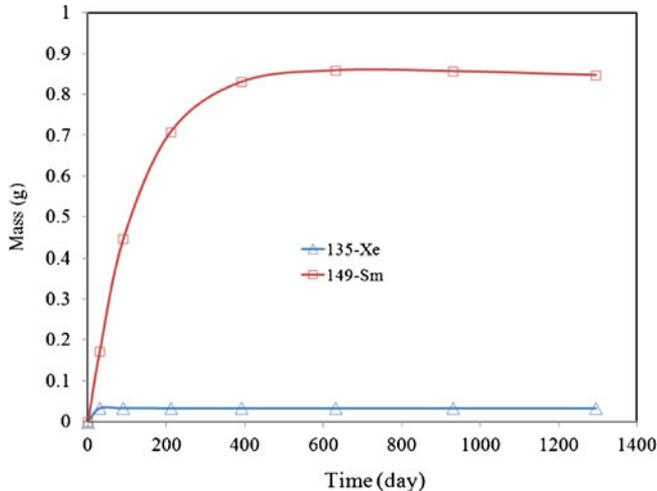
**Figure 14.** Xe and Sm accumulations vs. reactor operation time, BeO: 15 cm, core height: 140 cm, En: 2.2% of <sup>235</sup>U, gap between the assemblies: 0.5 cm.
