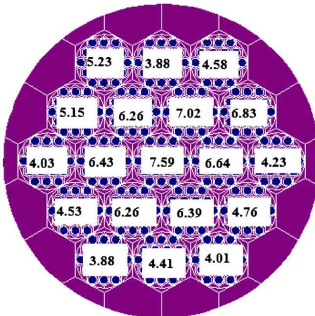
**Figure 10.** Normalized power distribution vs. arbitrary unit, BeO: 15 cm, core height: 140 cm, En: 2.2% of  $^{235}\text{U}$ , gap between the assemblies: 0.5 cm.
