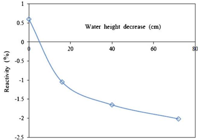
**Figure 9.** Void reactivity curve as a result of coolant circulation system failure, BeO: 15 cm, core height: 140 cm, En: 2.2% of  $^{235}\text{U}$ , gap between the assemblies: 0.5 cm.
