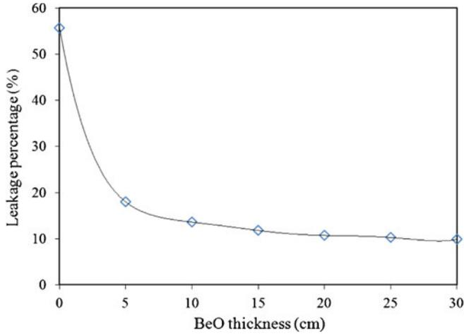
**Figure 6.** Core thermal neutron leakage percentage vs. reflector thickness variation. The gap between assemblies is 0.5 cm.
