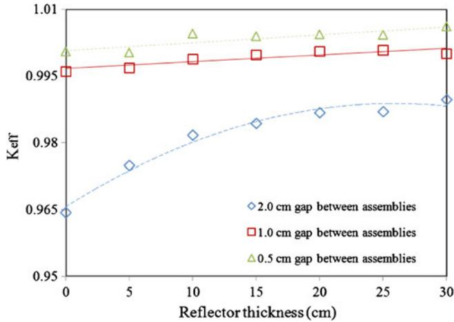
**Figure 4.** Comparison of  $K_{eff}$  with various reflector thicknesses. Gaps between assemblies are 2, 1 and 0.5 cm respectively.
