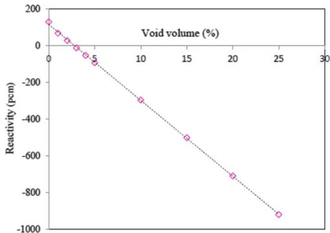
**Figure 17.** Void reactivity variations, BeO: 15 cm, core height: 140 cm, En: 2.2% of  $^{235}\text{U}$ , gap between the assemblies: 0.5 cm.
