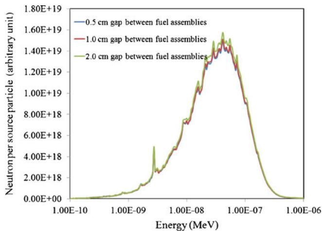
**Figure 2.** Comparison of core neutron spectra of various gaps between fuel assemblies.
