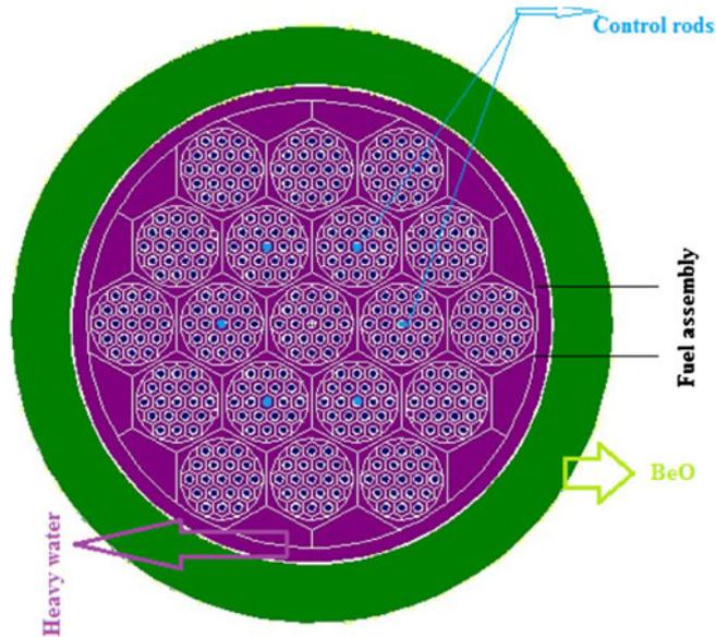
**Figure 1.** Critical core configuration consisting of 19-assemblies, a 15 cm thick BeO reflector and 2.2% (atom fraction) of  $^{235}\text{U}$ ; six silver alloy control rods of 2.08 cm diameter, 356 fuel rods of 2.08 cm diameter.
