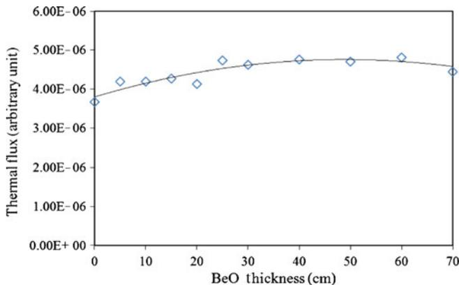
**Figure 5.** Core thermal flux variations vs. reflector thickness. The gap between assemblies is 0.5 cm.
