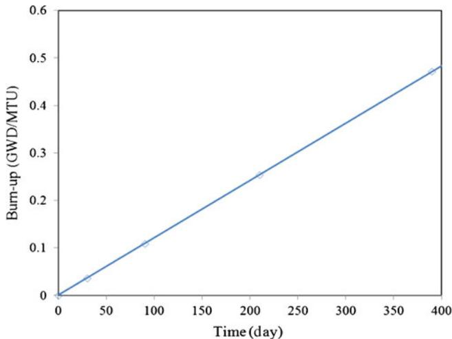
**Figure 12.** Burn-up, BeO: 15 cm, core height: 140 cm, En: 2.2% of  $^{235}\text{U}$ , gap between the assemblies: 0.5 cm.
