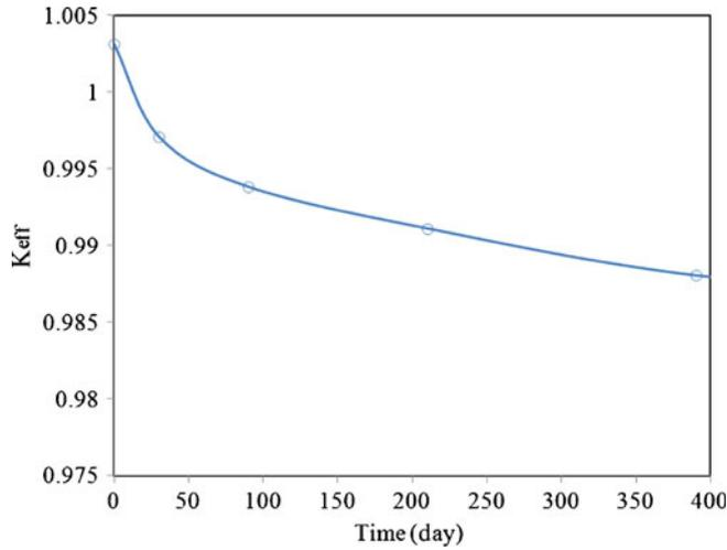
**Figure 11.** Multiplication on reactor operation time, BeO: 15 cm, core height: 140 cm, En: 2.2% of  $^{235}\text{U}$ , gap between the assemblies: 0.5 cm.
