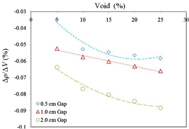
**Figure 8.** Void reactivity curve as a result of gas formation, BeO: 15 cm, core height: 140 cm, En: 2.2% of  $^{235}\text{U}$ .
