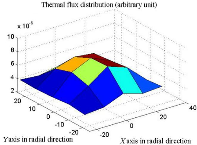
**Figure 7.** Core thermal neutron distribution vs. assembly position. The gap between assemblies is 0.5 cm.
