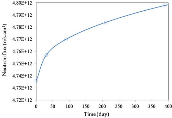
**Figure 13.** Neutron flux vs. operation time, BeO: 15 cm, core height: 140 cm, En: 2.2% of <sup>235</sup>U, gap between the assemblies: 0.5 cm.
