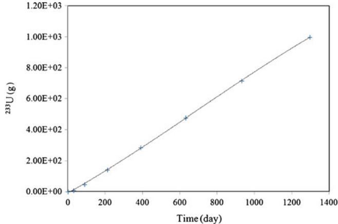
**Figure 15.** <sup>233</sup>U accumulation vs. reactor operation time, BeO: 15 cm, core height: 140 cm, En: 2.2% of <sup>235</sup>U, gap between the assemblies: 0.5 cm.
