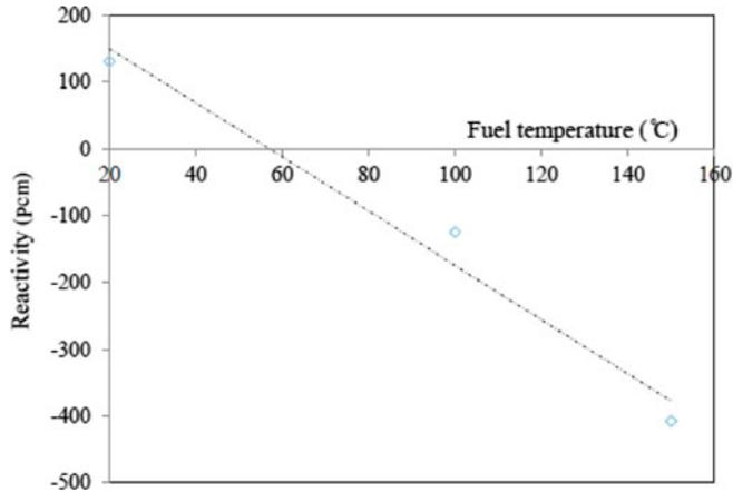
**Figure 16.** Fuel reactivity variations, BeO: 15 cm, core height: 140 cm, En: 2.2% of  $^{235}\text{U}$ , gap between the assemblies: 0.5 cm.
