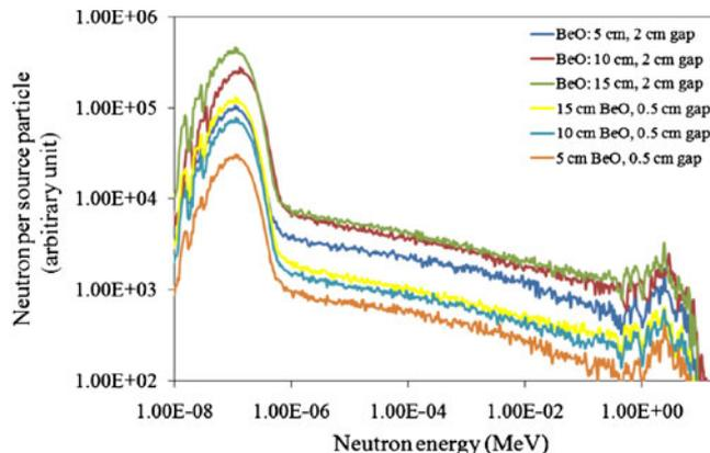
**Figure 3.** Comparison of reflector neutron spectra with various reflector thicknesses. Gaps between assemblies are 2 cm and 0.5 cm, respectively.
