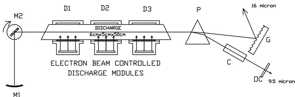
**Figure 1.** Schematic of the set-up for the 16  $\mu\text{m}$  laser. M1 – fully reflecting curved mirror of 10 m radius of curvature, M2 – fully reflecting rotating plane mirror, D1, D2, D3 – electron beam-controlled discharge modules, with discharge dimension 6 cm  $\times$  5 cm  $\times$  50 cm, P – KBr prism, G – 60 lines/mm grating with 85% efficiency, C –  $\text{SF}_6$  cell, OC – output coupler with 98% reflectivity.
