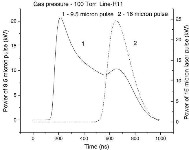
**Figure 9.** The calculated pulse shapes and amplitudes of the cascade laser.
