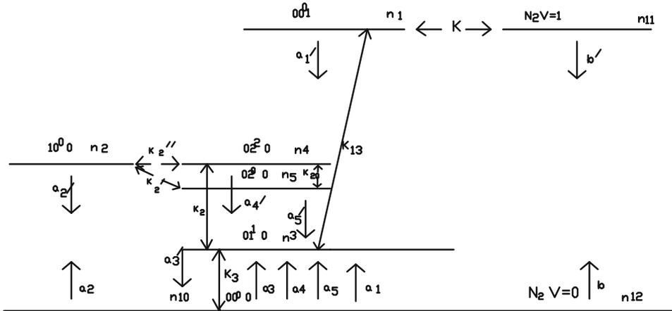
Figure 7. Energy level diagram of CO<sub>2</sub> laser.
