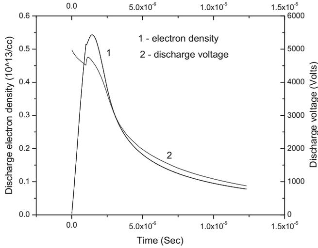
Figure 6. Variation of discharge voltage and electron density in the discharge with time.
