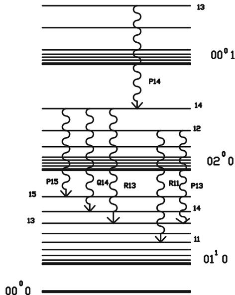
**Figure 8.** Energy level diagram of  $\text{CO}_2$  laser, showing rotational levels and cascade laser transitions.
