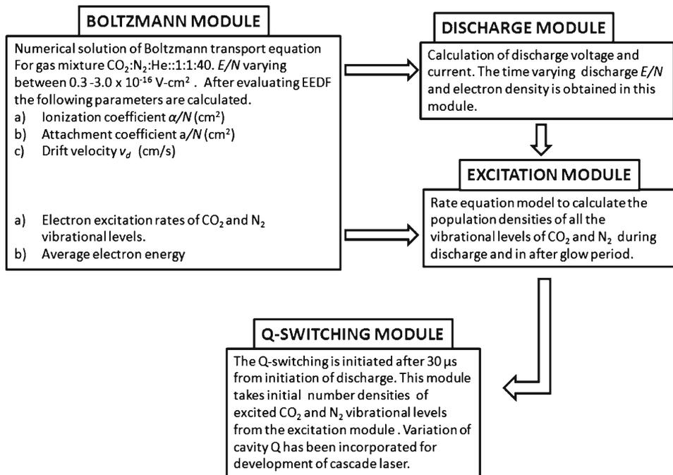
**Figure 2.** Simulation flow chart for calculating energy and power from cascade laser.
