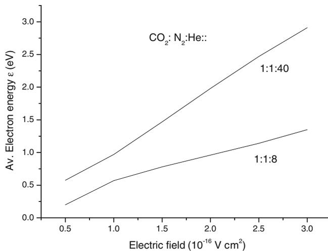
**Figure 5.** Variation of average electron energy ( $\epsilon$ ) with  $E/N$  for gas mixtures  $\text{CO}_2$ :  $\text{N}_2$ : He::1: 1: 8 and  $\text{CO}_2$ :  $\text{N}_2$ : He::1: 1: 40.
