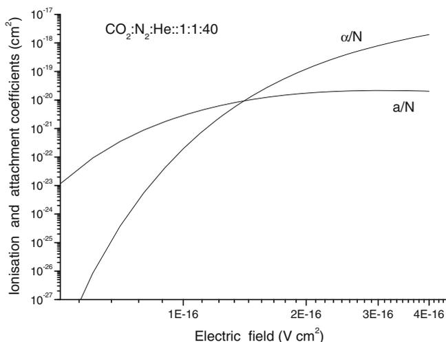
**Figure 3.** Variation of ionization coefficient ( $\alpha$ ) and attachment coefficient ( $a$ ) with  $E/N$ .
