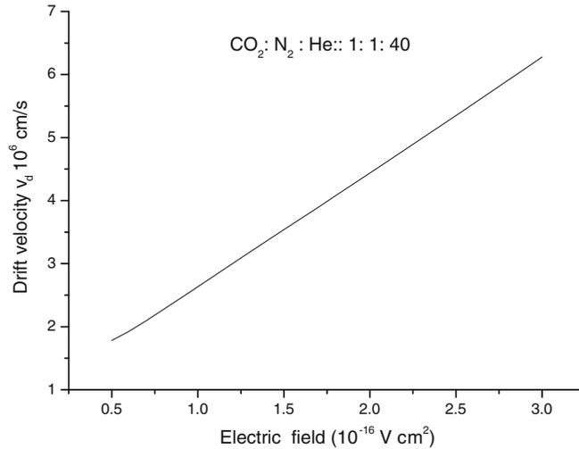
**Figure 4.** Variation of drift velocity ( $v_d$ ) with  $E/N$ .
