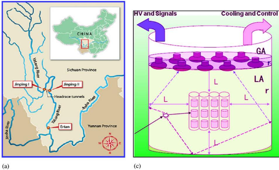
**Figure 2.** (a) Geographical location of CJPL, (b) the expected cosmic muon flux with respect to depth and (c) schematics of the proposed multiarray germanium detectors with liquid argon as anti-Compton veto at CJPL.
