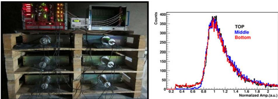
**Figure 3.** Cosmic ray muon set-up at CJPL with the calibration performed at sea level.
