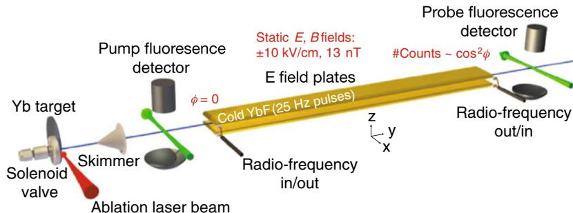
**Figure 7.** Sketch of the ICL YbF electron EDM experiment [42] (modified). Pulsed YbF molecules travel from the left to the right in between the electric field plates.
