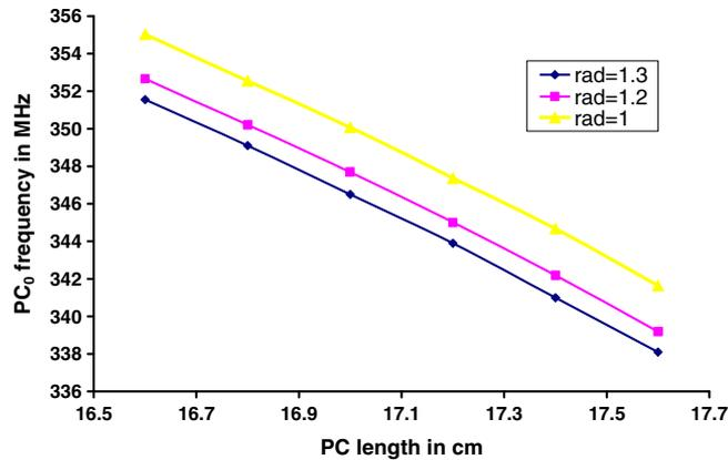
**Figure 12.** TE mode frequency as a function of post coupler length and radius.
