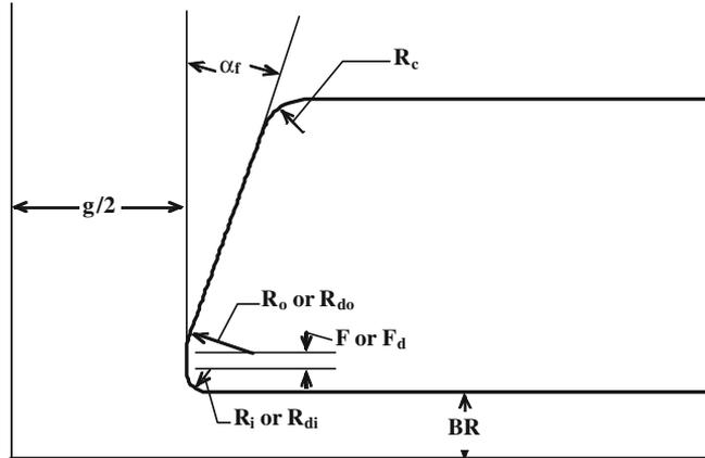
**Figure 3.** Detailed view of the drift tube.  $R_i$  – inner nose radius,  $R_c$  – corner radius and  $\alpha_f$  – face angle.
