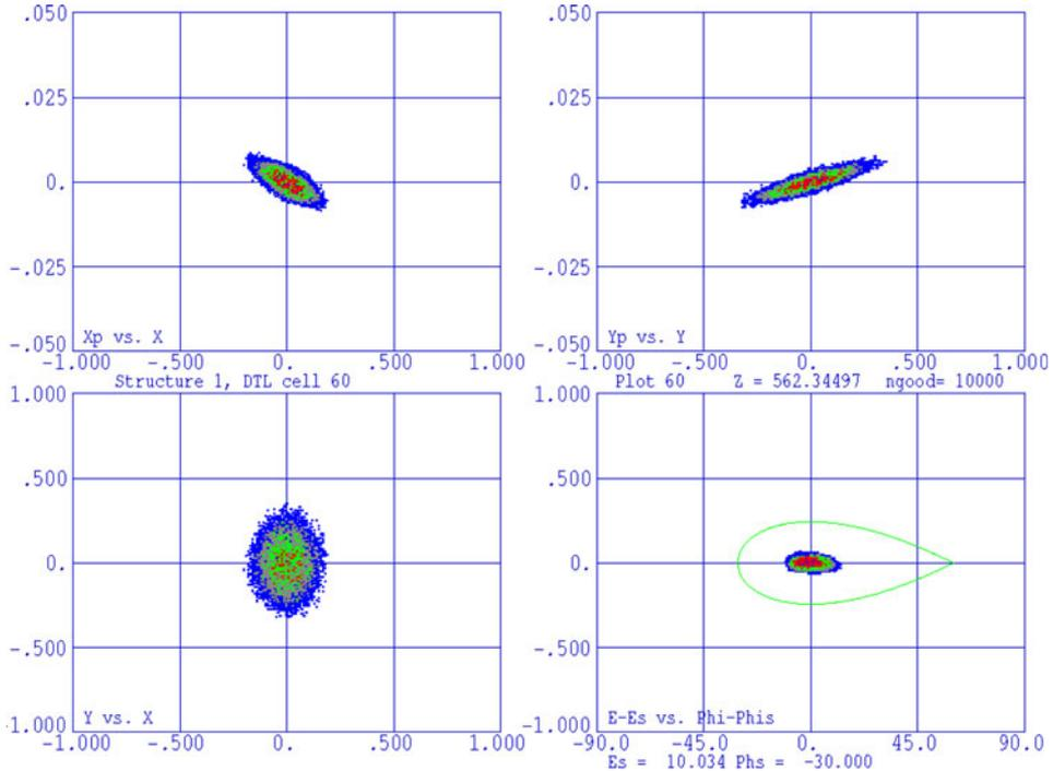
**Figure 6.** Phase space plots for  $x$  vs.  $x'$ ,  $y$  vs.  $y'$ ,  $x$  vs.  $y$  and  $E - E_s$  vs.  $\phi - \phi_s$  for the 60th cell.
