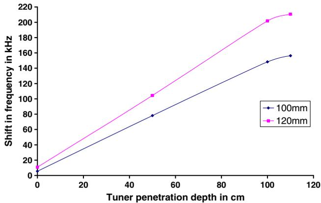
**Figure 10.** Tuner penetration depth vs. shift in resonant frequency.
