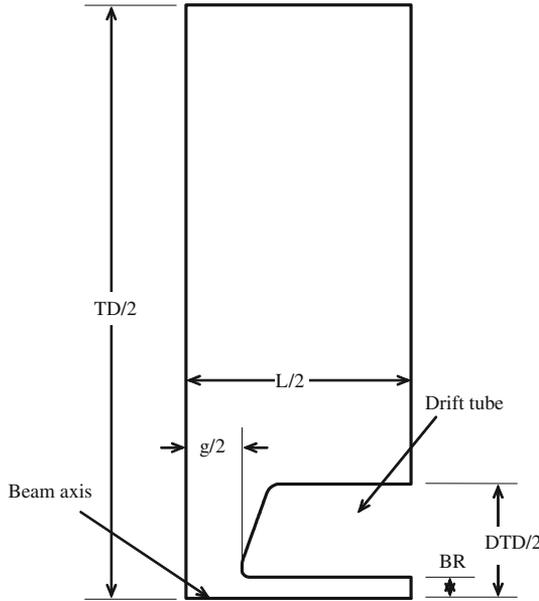
**Figure 2.** 1/4th unit cell drift tube geometry. TD – tank diameter, DTD – drift tube diameter, BR – bore radius, g – gap length, L – cell length.
