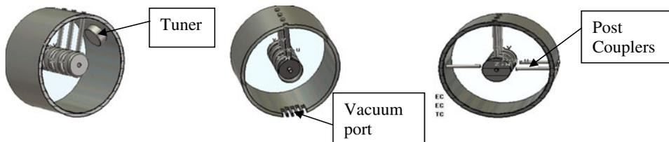
Figure 8. 3D Plots showing tuner, vacuum port and post couplers.
