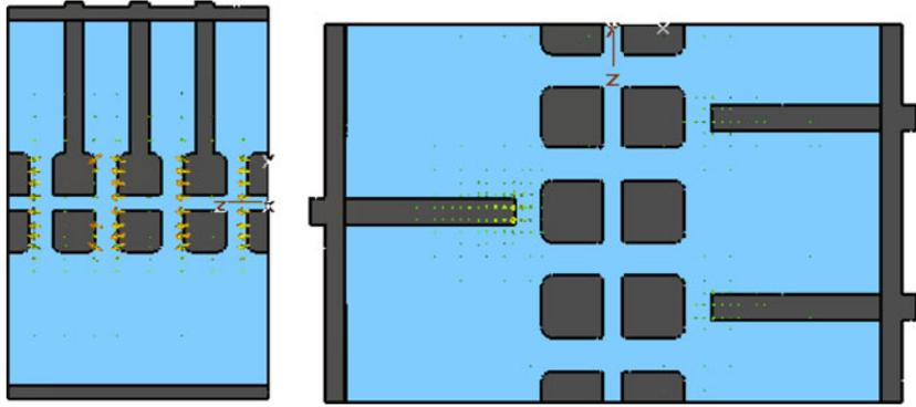
**Figure 9.** Field configuration for the fundamental mode and the post coupled mode.
