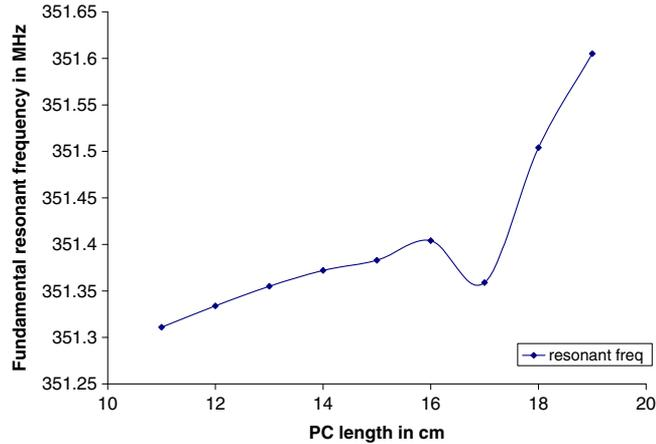
**Figure 11.** Resonant frequency vs. length of the post coupler for a post coupler radius of 1.3 cm.
