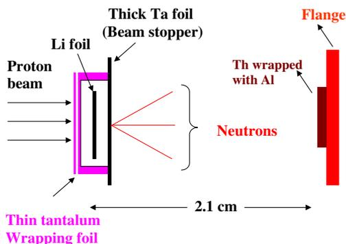
**Figure 1.** Schematic diagram showing the arrangement used for neutron irradiation.
