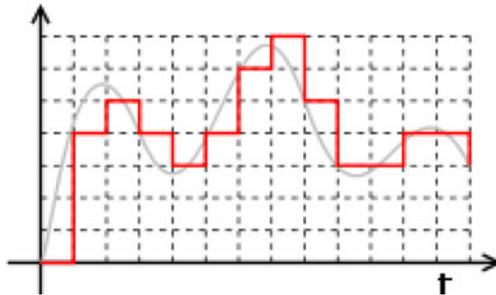
Figure 5. Digital signal (sampled, quantized): discrete time, discrete values.
