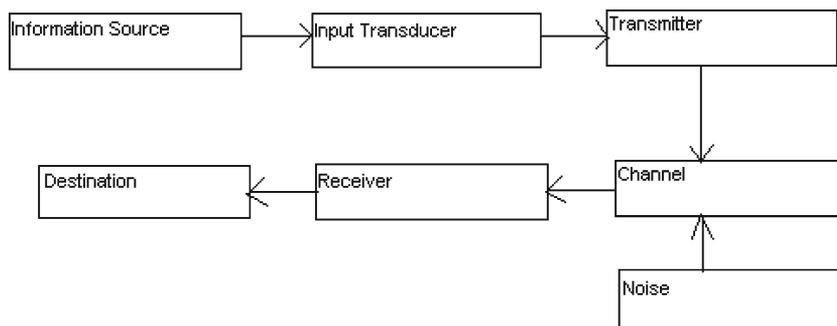
**Figure 1.** Basic communication system.
