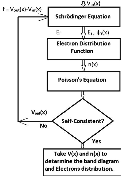
**Figure 3.** Flow chart showing the self-consistent solution of Poisson and Schrödinger equations in the  $\text{Al}_{0.3}\text{Ga}_{0.7}\text{N}/\text{GaN}$  HEMT structure.
