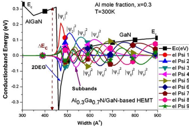
Figure 4. Formation of 2DEG with subbands for different electron eigenvalues.
