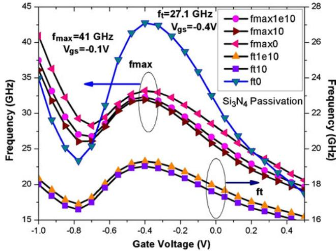
Figure 9. Maximum frequency of oscillation ( $f_{max}$ ) and cut-off frequency ( $f_t$ ) for Si<sub>3</sub>N<sub>4</sub> passivation.
