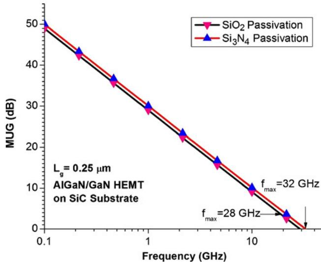
Figure 12. MUG for Si<sub>3</sub>N<sub>4</sub> and SiO<sub>2</sub> passivation layers showing unit power gain cut-off frequency.
