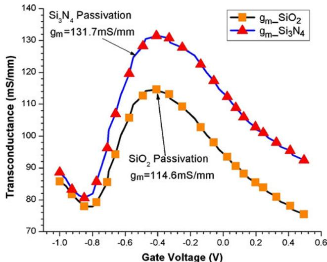
Figure 8. Extrinsic transconductance for  $\text{Si}_3\text{N}_4$  and  $\text{SiO}_2$  passivation layers.
