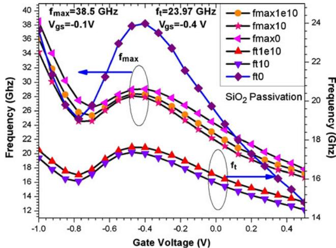
Figure 10. Maximum frequency of oscillation ( $f_{max}$ ) and cut-off frequency ( $f_t$ ) for SiO<sub>2</sub> passivation layer.
