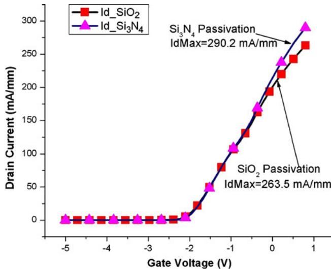
Figure 5. Gate characteristics for Si<sub>3</sub>N<sub>4</sub> and SiO<sub>2</sub> passivation layers.
