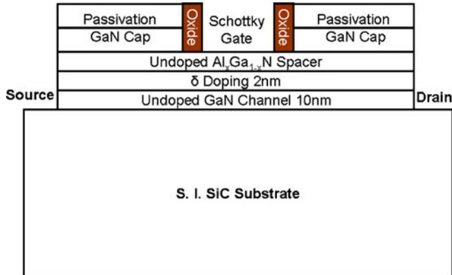
**Figure 1.** Simplified structure of the proposed AlGaN/GaN-based HEMT on SiC substrate.
