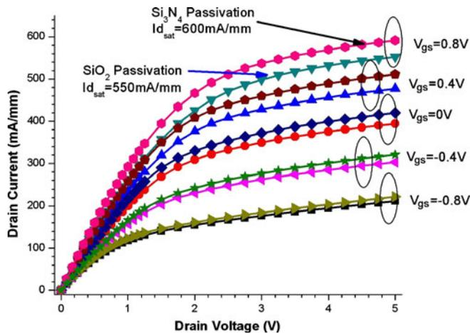
Figure 6. Drain characteristics for Si<sub>3</sub>N<sub>4</sub> and SiO<sub>2</sub> passivation layers.
