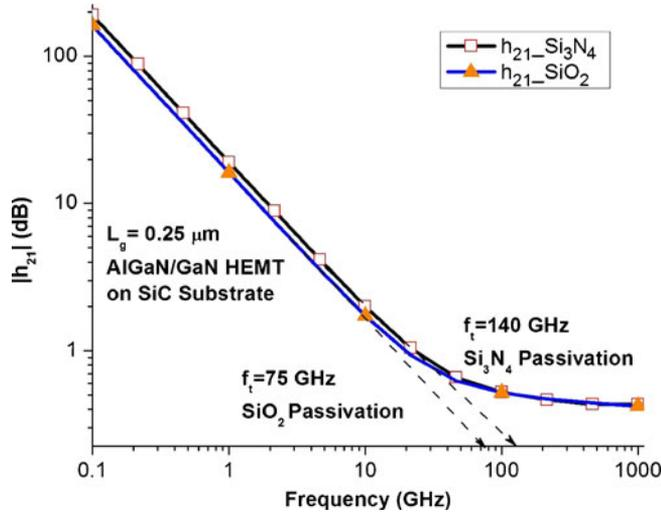
**Figure 13.** Abs  $|h_{21}|$  for  $\text{Si}_3\text{N}_4$  and  $\text{SiO}_2$  passivation layers showing unit current gain cut-off frequency.
