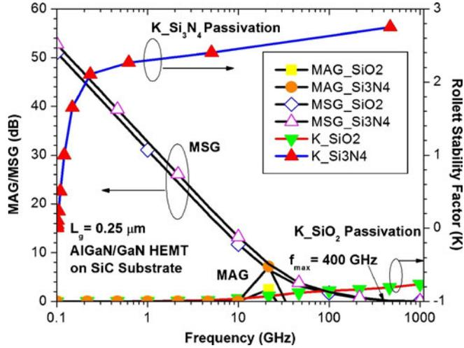
Figure 11. MAG/MSG for Si<sub>3</sub>N<sub>4</sub> and SiO<sub>2</sub> passivation layers showing the stability.
