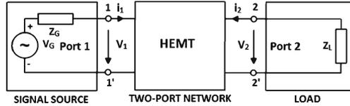
Figure 7. HEMT in two-port network.
