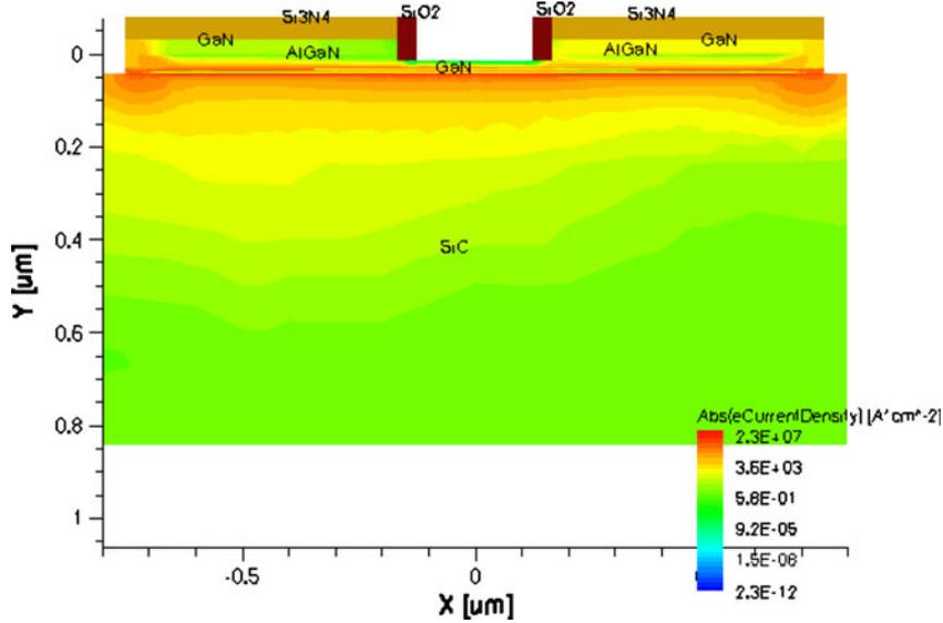
**Figure 2.** Simulated structure of the proposed AlGaIn/GaN-based HEMT on SiC substrate.
