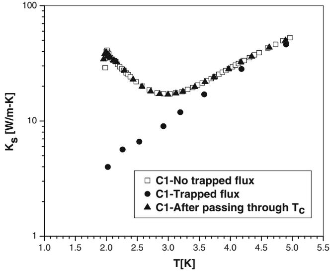
**Figure 12.** Plot of thermal conductivity in superconducting state in zero remnant field, with remnant field and heating up the sample through  $T_c$  to exclude the flux lines to reproduce the zero-field curve.
