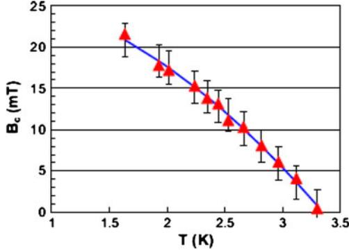
**Figure 2.** Critical magnetic field as a function of temperature measured on an indium rod of 99.99% purity. The solid line is a least-square fit with eq. (3).
