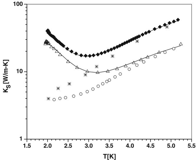
**Figure 7.** Plot of  $K_S$  vs.  $T$ . (■) C1 – zero field, (\*) C1 – trapped flux 81 mT, ( $\Delta$ ) A1 – zero field, (o) A1 – trapped flux 60 mT. Solid lines are the fitting curves of eq. (6).
