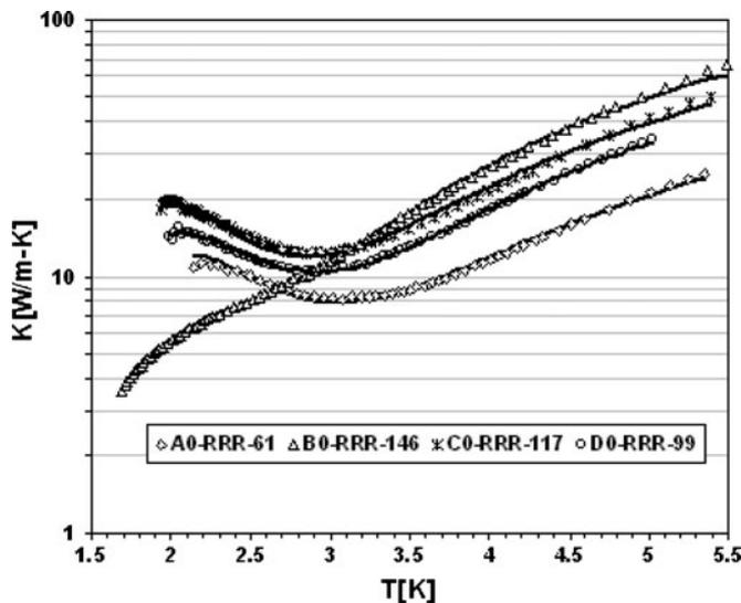
**Figure 4.** Experimental thermal conductivity data for  $180 \mu\text{m}$  buffered chemical polished niobium samples from four different ingots. Solid lines are the fitting curves.
