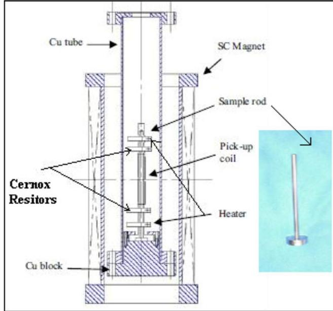
**Figure 1.** Schematic of the system for measuring the superconducting properties of the sample and a picture of the sample rod.
