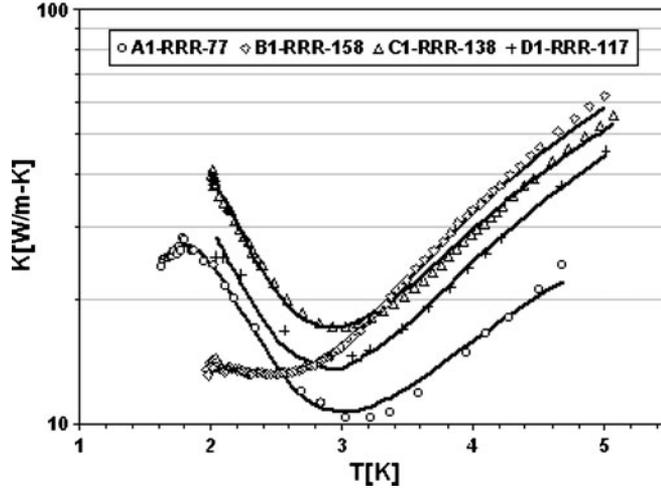
**Figure 5.** Experimental thermal conductivity data for 600°C heat treated niobium samples from four different ingots. Solid lines are the fitting curves.
