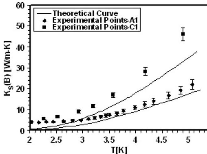
**Figure 9.** Effect of trapped vortices on the thermal conductivity of the superconducting state in samples A1 and C1. Solid lines represent the qualitative theoretical model by Vinen *et al* at low inductions and low temperature.
