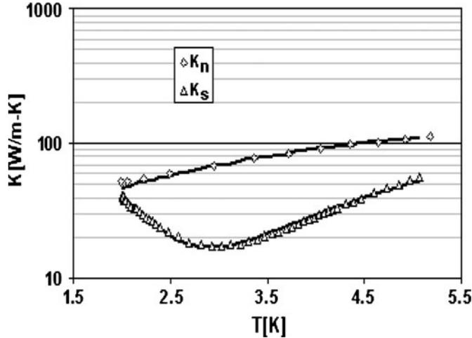
**Figure 6.** Thermal conductivity data in normal and superconducting states for the sample C1. Solid lines are the fitting curves with eq. (6).
