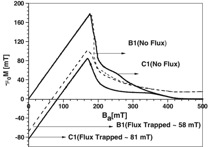
**Figure 8.** Magnetization curves at  $T = 2$  K with and without remnant magnetization for (—) A1, (---) C1.
