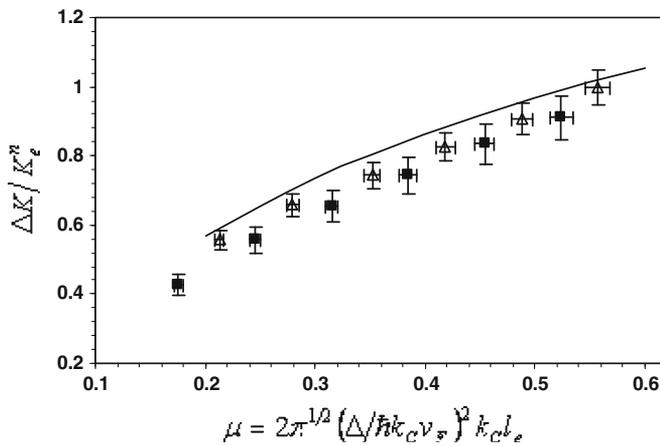
**Figure 11.**  $\Delta K/K_e^n$  as a function of  $\mu$  in sample B1. ( $\Delta$ ) Sample B1 without any trapped flux in zero field, ( $\blacksquare$ ) sample B1 with an initial remnant magnetization of about 58 mT. Solid line is the theoretical curve of Houghton–Maki.
