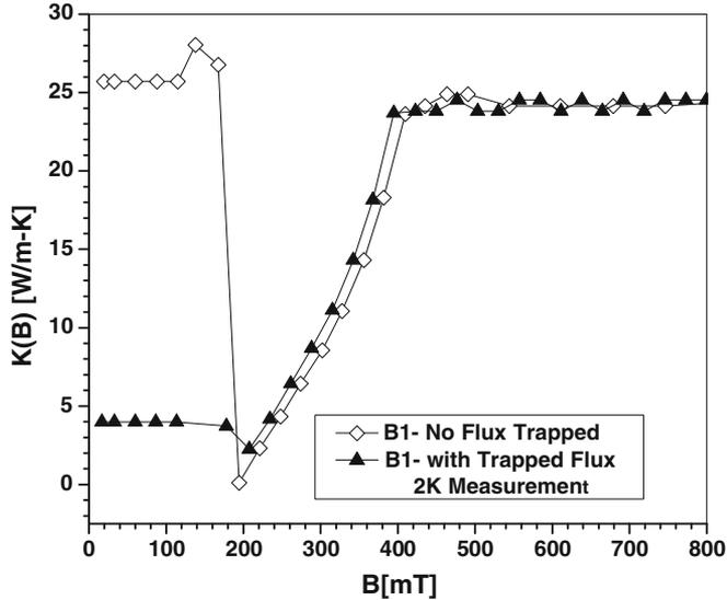
**Figure 10.** Field dependence of the thermal conductivity with and without trapped vortices measured with the field parallel to the heat flow direction at 2 K.
