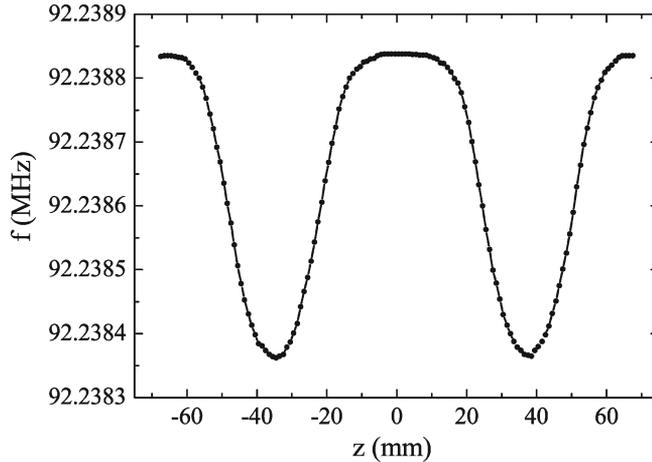
**Figure 16.** Frequency as a function of the bead position when a spherical dielectric bead is pulled through the beam axis of the resonator.
