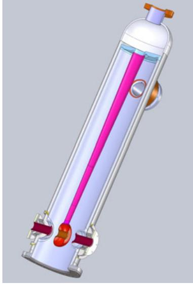
**Figure 15.** Cut away 3D view of the low beta resonator design showing niobium components inside and the stainless steel vessel outside.
