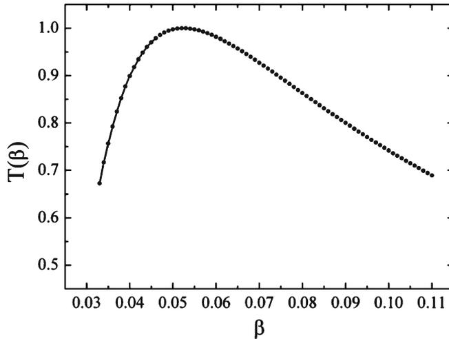
**Figure 13.** Transit time factor as a function of  $\beta$  for the final design of the low beta resonator.
