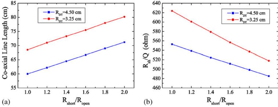
**Figure 8.** (a) Length of the coaxial line  $L_{\text{CC}}$  and (b) geometric shunt impedance  $R_{\text{sh}}/Q$ , as a function of the ratio of the radii at the end of the coaxial line, for the two different drift tubes.
