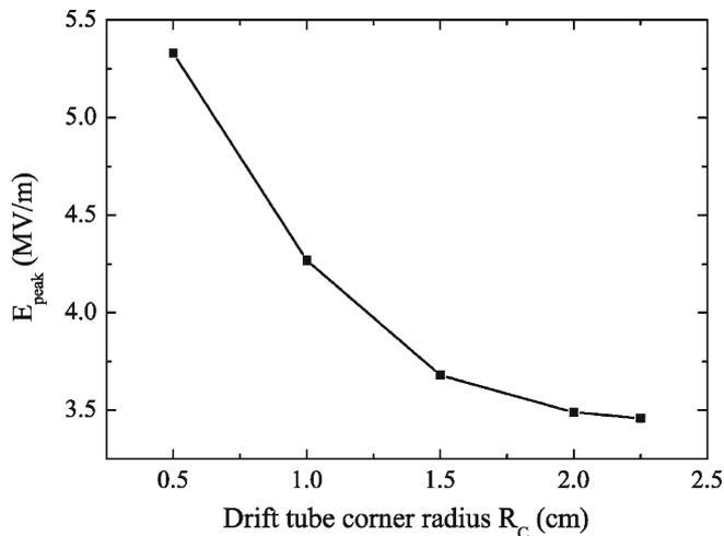
**Figure 12.** Peak surface electric field at 1 MV/m accelerating gradient as a function of drift tube corner radius  $R_C$ .
