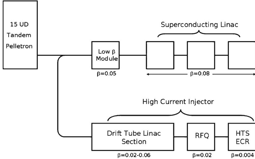
**Figure 1.** Block diagram of the proposed high current injector (HCI) system at IUAC.
