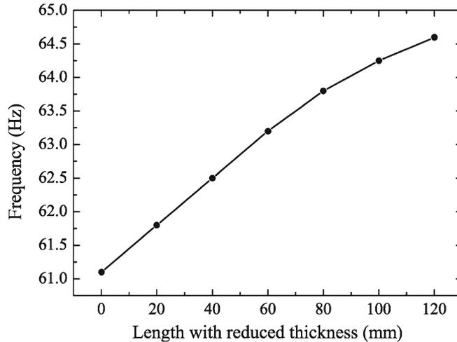
**Figure 14.** Frequency of the lowest mechanical eigenmode as a function of the length over which the wall thickness of the central coaxial line is reduced from 3 to 1.5 mm.
