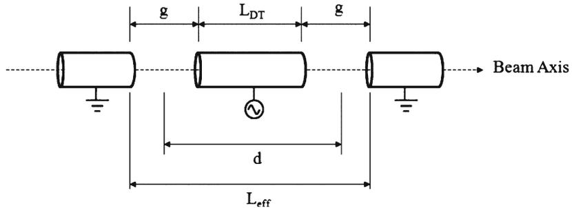
**Figure 2.** Schematic diagram of a two-gap accelerating system. The drift tube of length  $L_{DT}$  is in the middle. The two tubes at either end of the drift tube are the ports on the outer housing. The acceleration takes place in the two gaps (each of length  $g$ ).
