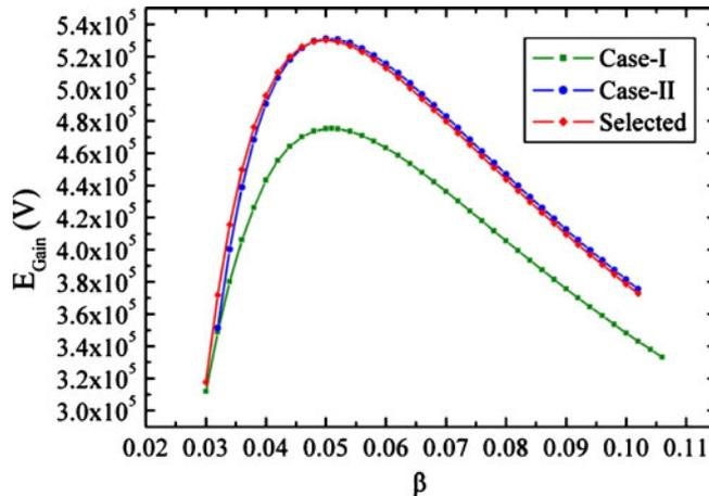
**Figure 4.** Energy gain per charge state vs. beta for the two cases shown in table 1. For comparison the final set selected for the design is also shown. The calculations are shown for 1 J of stored energy in the resonator.
