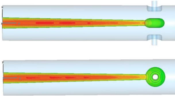
**Figure 9.** MWS output of the  $x$ - and  $y$ -components of the magnetic field along the tapered coaxial line, for the drift tube of radius  $R_{DT} = 4.50$  cm.
