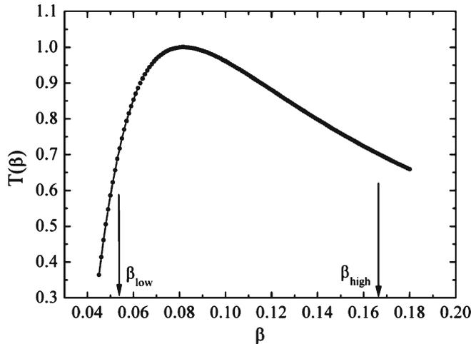
**Figure 3.** Transit time factor  $T(\beta)$  vs.  $\beta$  for the quarter-wave resonators installed in the superconducting Linac. The two velocities  $\beta_{\text{high}}$  and  $\beta_{\text{low}}$  indicate the range for which the energy gain is more than 70% of the maximum.
