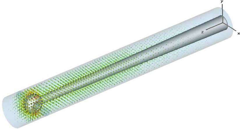
**Figure 6.** Results of calculations using Microwave Studio model showing the transverse electric field along the coaxial line, for the drift tube of radius  $R_{DT} = 3.25$  cm.
