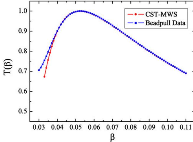
**Figure 18.** Comparison of transit time factor as a function of  $\beta$  calculated from the bead pull data with the results from MWS calculations.
