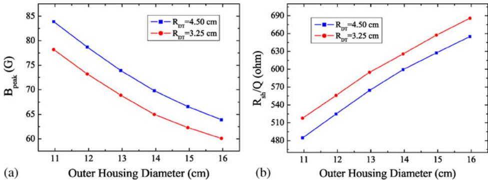
**Figure 10.** (a) Peak magnetic field and (b) geometric shunt impedance, as a function of outer housing diameter for  $(R_{short}/R_{open}) = 2$ , for the two different drift tubes.
