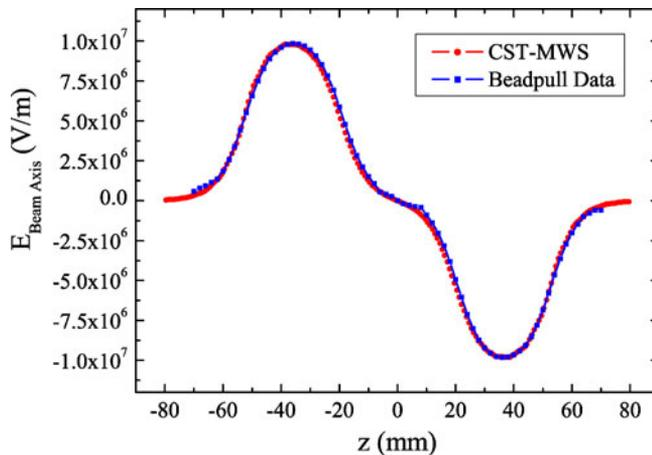
**Figure 17.** Electric field profile along the beam axis of the copper model of the resonator. For comparison, data from Microwave Studio calculations are also shown.
