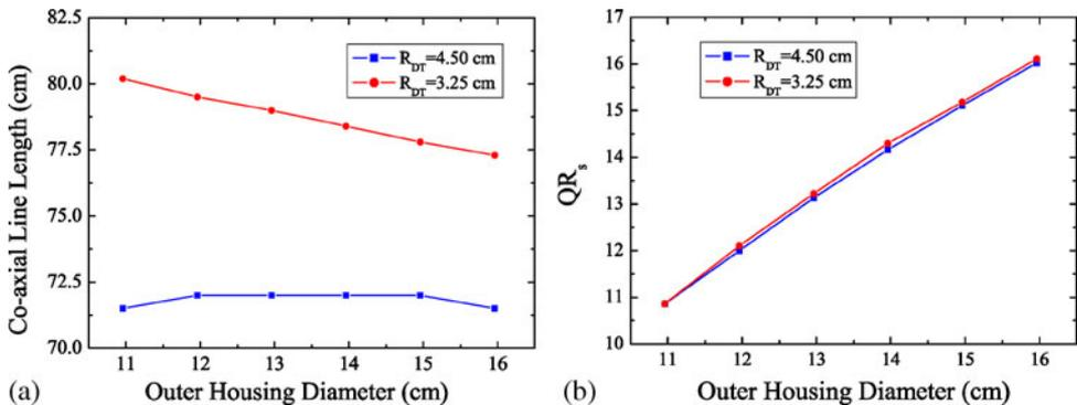
**Figure 11.** (a) Coaxial line length  $L_{CC}$  and (b) geometry factor  $QR_s$ , as a function of the outer housing diameter for  $(R_{short}/R_{open}) = 2$ , for the two different drift tubes.
