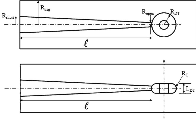
**Figure 5.** Schematic diagram of a linearly tapered coaxial line quarter-wave resonator. The upper and lower diagrams show the view in two perpendicular planes. The drift tube is attached at the end of the central tapered coaxial line. The dashed line with arrow through the drift tube in the lower figure indicates the beam axis, which is perpendicular to the plane of the paper in the upper figure.
