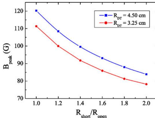
**Figure 7.** Peak magnetic field as a function of the ratio of the radii at the two ends of the coaxial line, for the two different drift tubes.
