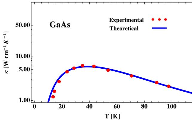
Figure 6. Analysis of thermal conductivity of GaAs (sample III).
