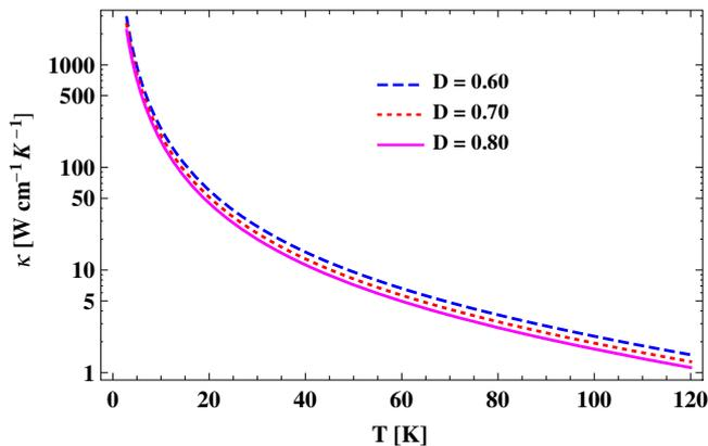
**Figure 3.** Influence of interference scattering on thermal conductivity.
