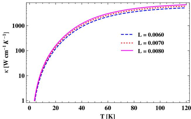
**Figure 1.** Effect of the scattering length of combined boundaries on lattice thermal conductivity.
