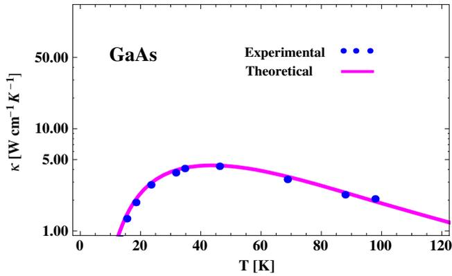
Figure 5. Analysis of thermal conductivity of GaAs (sample II).
