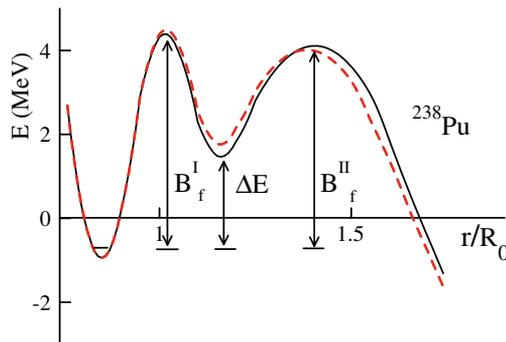
**Figure 4.** Calculated double-humped fission barrier on the basis of the combined dynamical–statistical model (solid curve) and the statistical model (dashed curve) for  $^{238}\text{Pu}$ .
