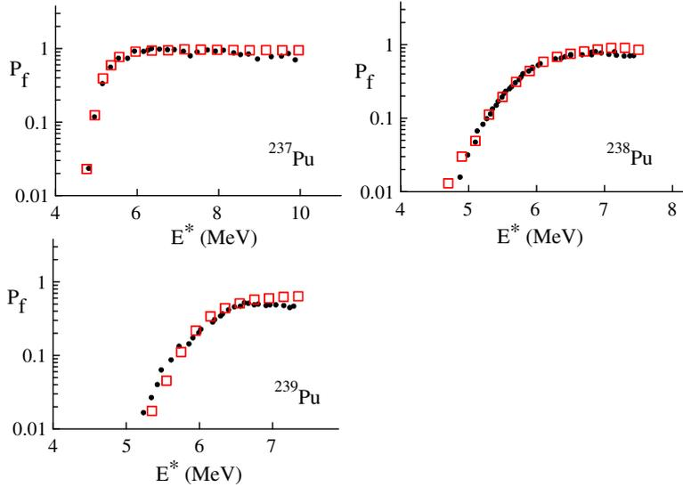
**Figure 2.** Fission probabilities of  $^{239}\text{Pu}$ ,  $^{238}\text{Pu}$  and  $^{237}\text{Pu}$ . ( $\square$ ) Calculation, ( $\bullet$ ) experimental data [19–21].
