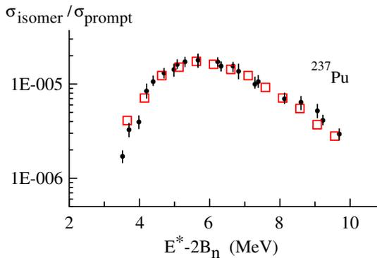
**Figure 3.** Yield of the  $^{237}\text{Pu}$  shape isomer for the  $\alpha + ^{235}\text{U}$  reaction. ( $\square$ ) Calculation, ( $\bullet$ ) experimental data [2].
