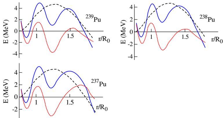
**Figure 1.** Calculated double-humped fission barrier (solid curve), liquid-drop fission barrier (dashed curve) and shell correction (dotted curve) for  $^{239}\text{Pu}$ ,  $^{238}\text{Pu}$  and  $^{237}\text{Pu}$ .  $R_0$  is the radius of the spherical nucleus.
