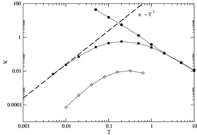
**Figure 2.** KG chain:  $\kappa(T)$  for  $W = 2$  (filled squares). For comparison we also show the data for  $\tilde{\epsilon}_l \equiv 1$  (filled circles). Thin solid lines guide the eye. The dashed line corresponds to the power law  $T^2$ . The stronger disorder case  $W = 6$  corresponds to the open diamond data points.
