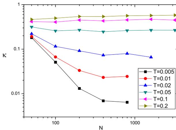
**Figure 1.** KG chain: the size-dependent thermal conductivity  $\kappa_N$  vs.  $N$  for different temperatures and  $W = 2$ .
