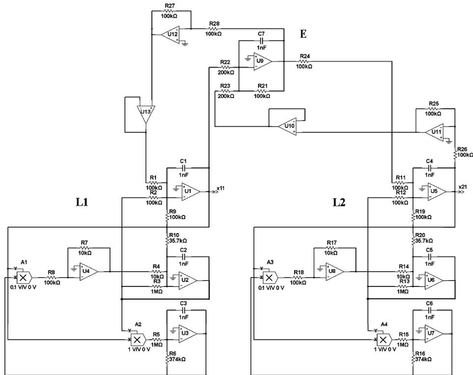
**Figure 1.** Schematic diagram of two indirectly coupled Lorenz electronic circuits for in-phase synchronization corresponding to eq. (2). All resistances (with 5% tolerance) are metallic and capacitors (with 1% tolerance) are ceramic. The circuit is run by  $\pm 12$  V.
