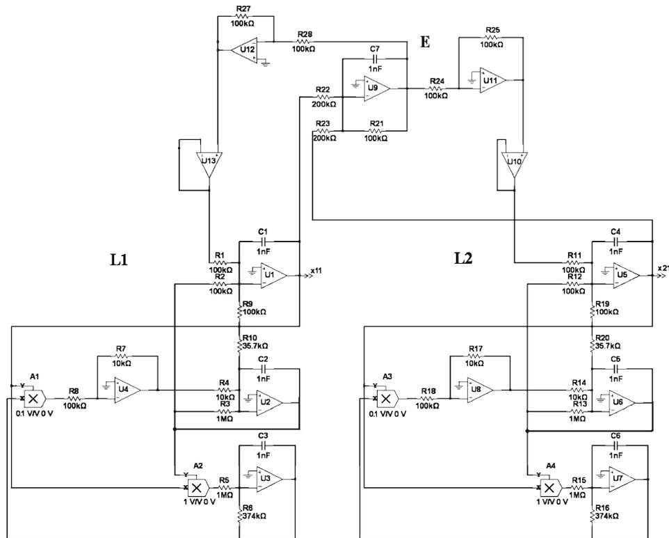
**Figure 2.** Schematic diagram of two indirectly coupled Lorenz electronic circuits for anti-phase synchronization corresponding to eq. (3). All resistances (with 5% tolerance) are metallic and capacitors (with 1% tolerance) are ceramic. The circuit is run by  $\pm 12$  V.
