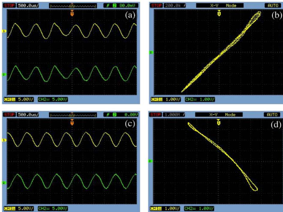
**Figure 5.** Time series and phase relationship of the two state variables of indirectly coupled piece-wise Rössler systems showing (a, b) in-phase and (c, d) anti-phase synchronizations.
