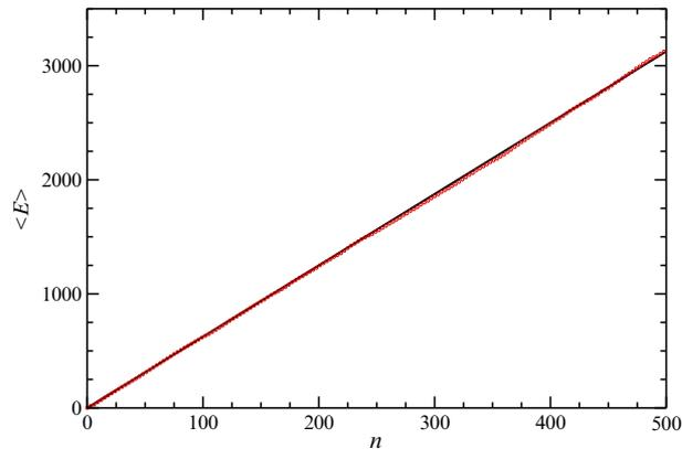
**Figure 6.** Growth in mean energy (open circles, red) as a function of time  $n$  for kick strength  $\epsilon = 5$  obtained from simulations. The other parameters are the same as in figure 5a. The black solid line corresponds to the analytical result  $\langle E \rangle = (\epsilon^2/4)n$  for the kicked rotor.
