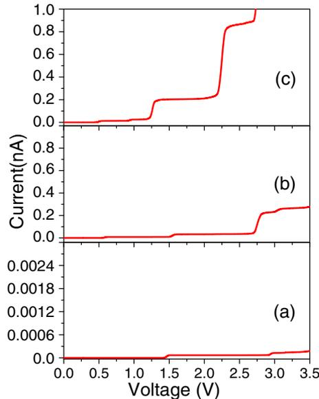
**Figure 3.** (a)–(c) panels show the  $I$ – $V$  characteristics of (10,0) BCN alloy nanotube for 20, 50 and 80% concentration of C atoms, respectively.
