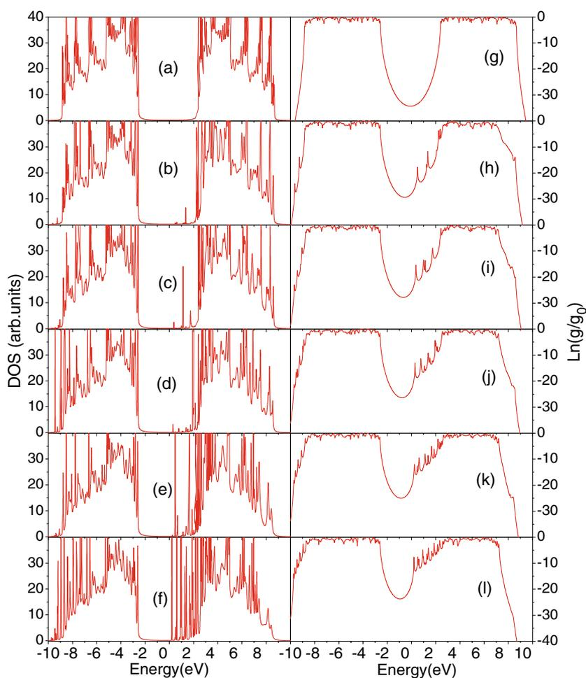
**Figure 2.** (a)–(f) panels show the DOS vs. energy for the BN and BCN nanotubes with 30, 40, 50, 60 and 70% concentration of C atoms, respectively. The nanotube is from (10,0) zig-zag type to the nearly 5.92 nm length. (g)–(l) panels show the conductance logarithm vs. energy that correspond to the (a)–(f) panels.
