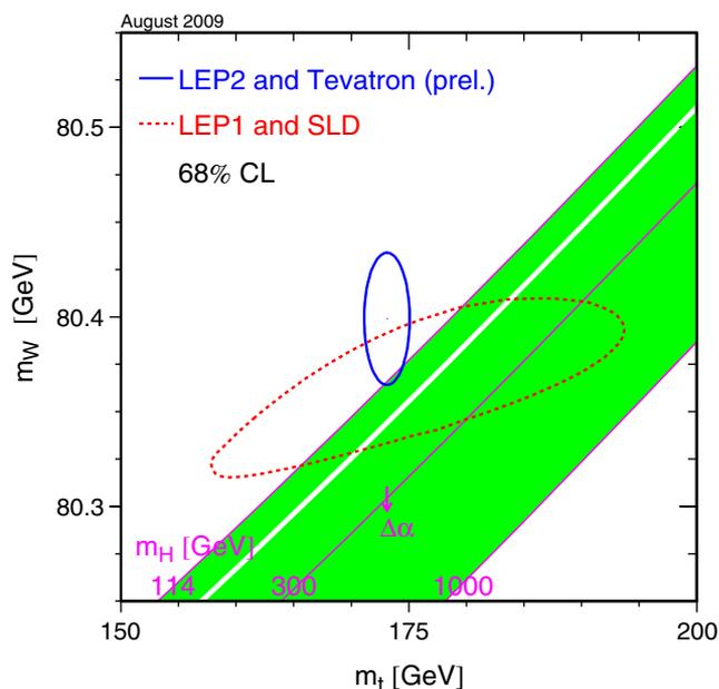
Figure 1. Mass constraint on a Standard Model Higgs boson from  $M_W$  and  $M_t$ .
