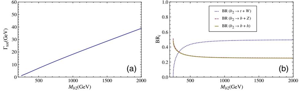
**Figure 5.** Total width (a) and BR (b) of  $b_2$  versus  $M_{b_2}$ . In figure 5b, the  $bZ$  and  $bh$  decay channel curves are almost on top of each other.
