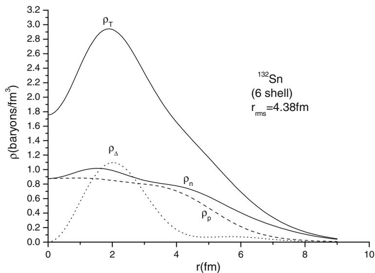
**Figure 4.** Total  $\rho_T$ , proton  $\rho_p$  (dashed line), neutron  $\rho_n$  (solid line) and delta  $\rho_\Delta$  (dotted line) radial density distributions for  $^{132}\text{Sn}$  at  $r_{\text{rms}} = 4.38$  fm in a model space of six major oscillator shells.
