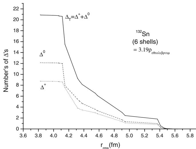
**Figure 2.** Number of  $\Delta$ s as a function of  $r_{\text{rms}}$  for  $^{132}\text{Sn}$  in six major shell model spaces. The upper curve indicates the total number of  $\Delta$ s, the dotted curve indicates the number of  $\Delta^+$ , and the dashed curve indicates  $\Delta^0$ .
