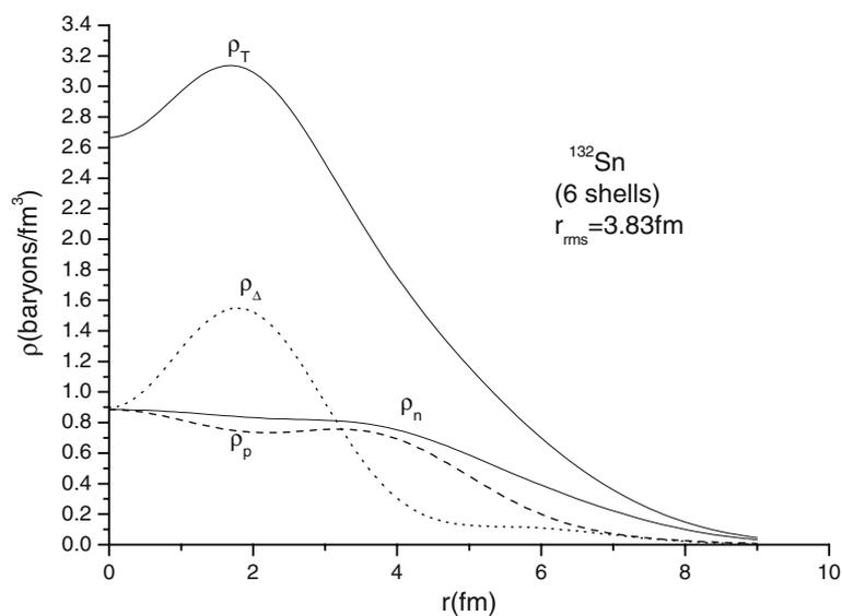
**Figure 5.** Total  $\rho_T$ , proton  $\rho_p$  (dashed line), neutron  $\rho_n$  (solid line) and delta  $\rho_\Delta$  (dotted line) radial density distributions for  $^{132}\text{Sn}$  at  $r_{\text{rms}} = 3.83$  fm in a model space of six major oscillator shells.
