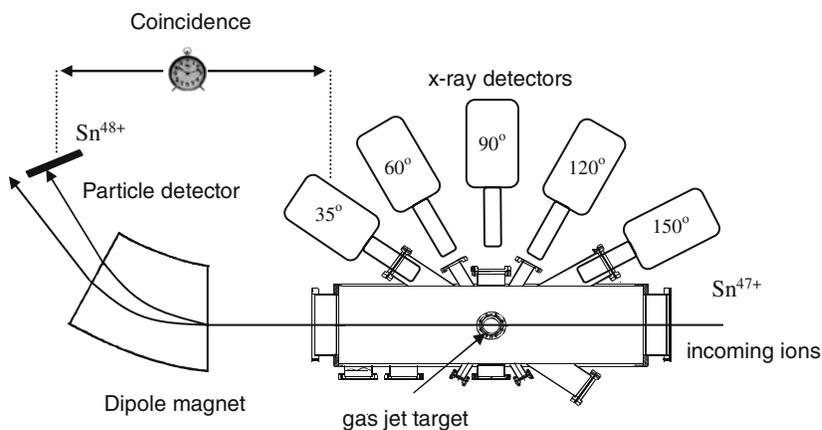
**Figure 2.** Lay-out of the experimental set-up at the internal jet target. X-ray detectors view the target interaction zone at different observation angles. Photon emission was observed in coincidence with the up-charged ions, detected in the particle counter located behind the dipole magnet.
