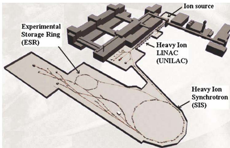
**Figure 1.** Lay-out of the accelerator facility and experimental areas at GSI, Darmstadt.
