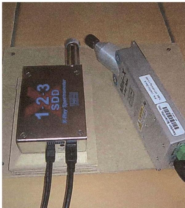
**Figure 1.** Portable EDXRF equipment, composed of a mini-X-ray tube with Ag anode, working at 40 kV maximum voltage and 100  $\mu\text{A}$  current, and of a 123Si-drift detector. Both X-ray tube and detector are manufactured by AMPTEK Inc. Bias supply for the X-ray tube is inserted in the X-ray tube case; both amplification circuits and pulse height analyser are in the 123 module [1].
