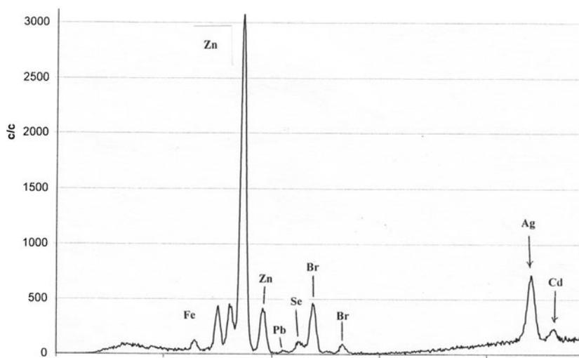
**Figure 3.** X-ray spectrum of the red area of the painting supposed to be of Giorgio De Chirico. The presence of Cd–Se red, which was never employed by De Chirico, at least in the period in which the painting was supposed to be made, supports the hypothesis that the painting is a fake.
