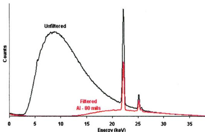
**Figure 2.** X-ray spectrum of a mini-X Ag anode X-ray tube at 40 kV, unfiltered and filtered (red curve) with 2 mm Al. For analysis of elements, for example Ag or Sn, only the last part of the spectrum is useful for excitation. The unfiltered first part only contributes to the background.
