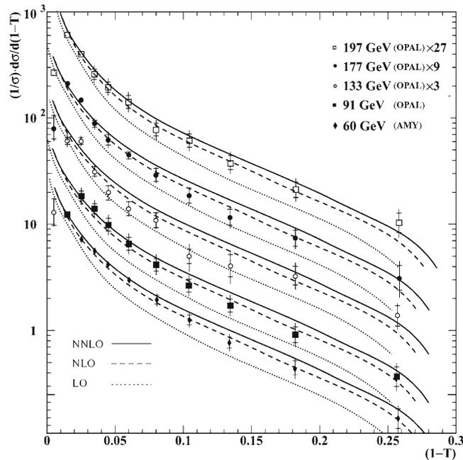
**Figure 4.** The thrust distribution at LO (dotted line), NLO (dashed line) and NNLO (solid line) compared to experimental data from AMY and OPAL for  $Q = 60$ – $197$  GeV. The data are from refs [7,10,11] and the model is from refs [1–3,12].
