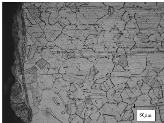
**Figure 8.** Microstructure in dry laser cutting of SS304 using oxygen.
