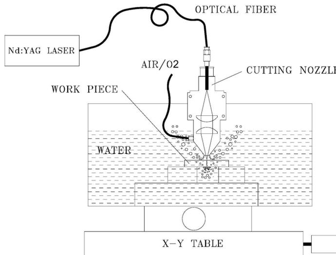
**Figure 1.** Experimental set-up for underwater laser cutting.
