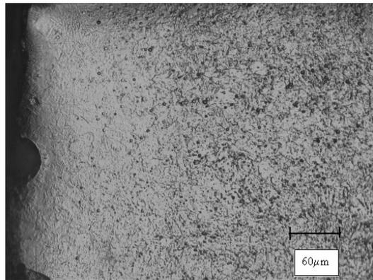
**Figure 5.** Microstructure in underwater laser cutting of zirconium alloy using air.
