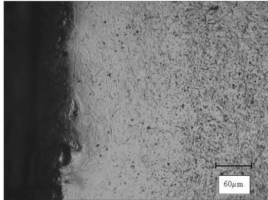
**Figure 6.** Microstructure in dry laser cutting of zircaloy using air.
