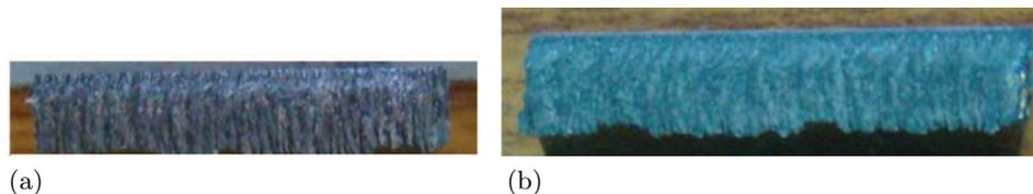
**Figure 3.** (a) Underwater laser cut surface of zircaloy using air. (b) Laser cut surface of zircaloy in dry condition using air.
