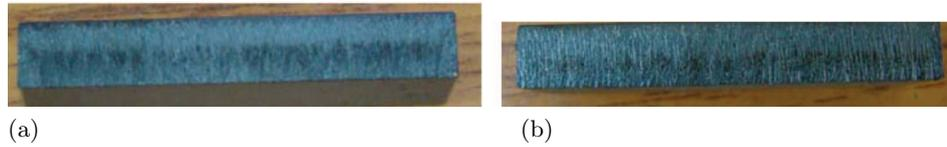
**Figure 4.** (a) Underwater laser cut surface of SS304 using oxygen. (b) Laser cut surface of SS304 in dry condition using oxygen.
