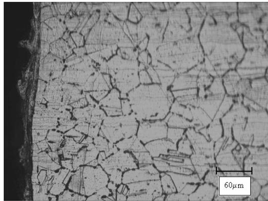
**Figure 7.** Microstructure in underwater laser cutting of SS304 using oxygen.
