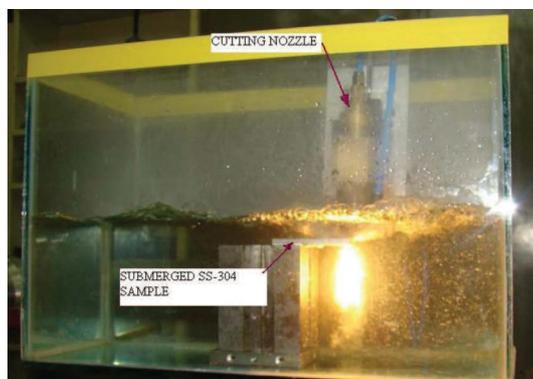
**Figure 2.** A view of the underwater laser cutting of SS304.
