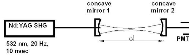
Figure 1. CRD set-up for measuring reflectivity of test mirror at  $0^\circ$  AOI.
