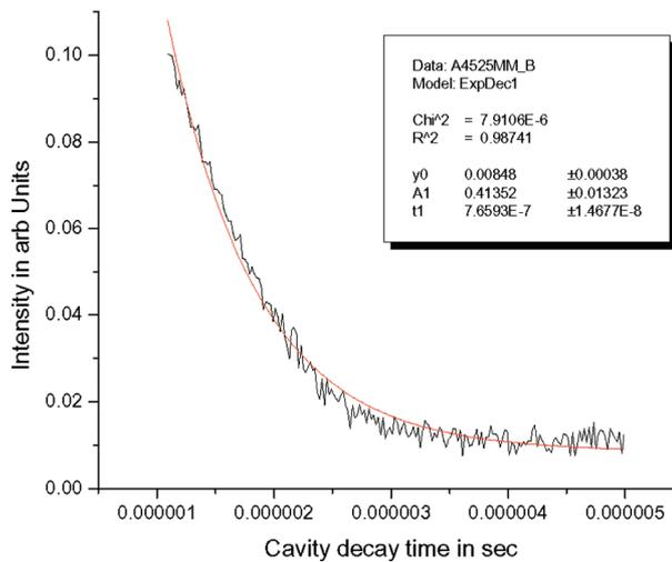
Figure 7. Exponential fitting results for L-shaped cavity containing the test mirror of 45° AOI.
