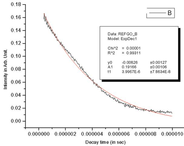
Figure 6. Exponential fitting of decay curve for the reference mirror.
