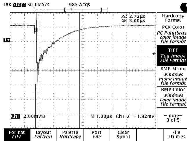
Figure 2. CRD signal as seen by the oscilloscope.
