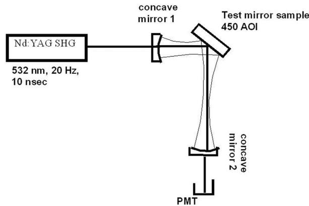
Figure 4. CRD set-up for measuring reflectivity of the test mirror at 45° AOI.
