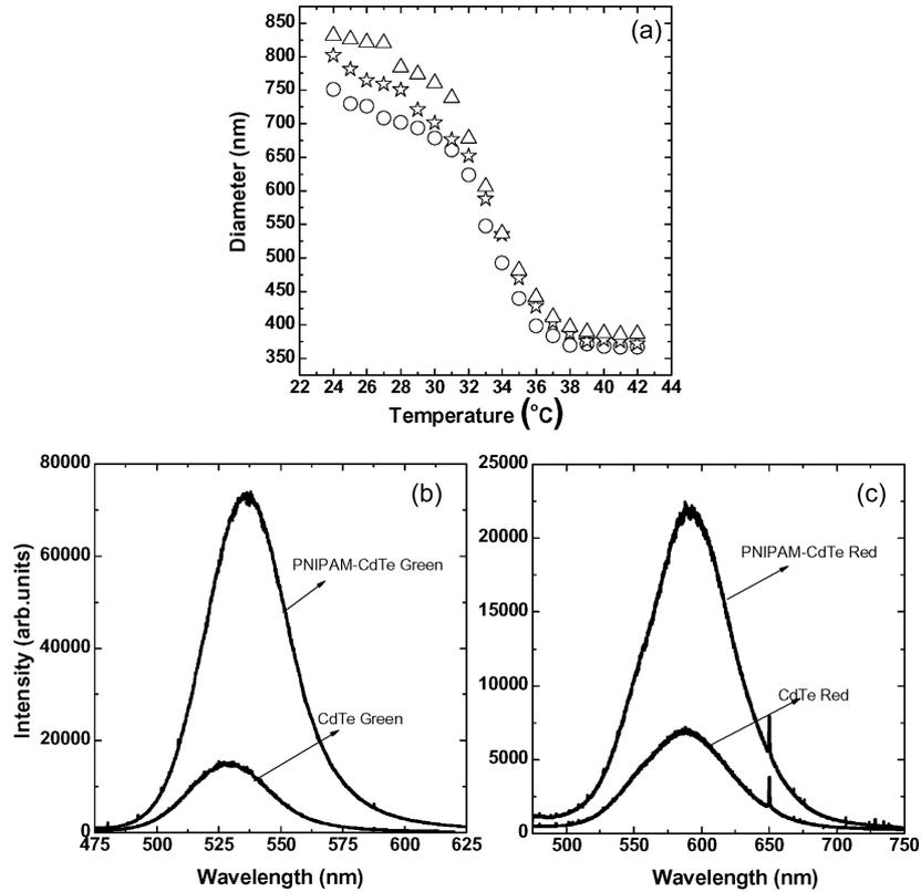
**Figure 1.** (a) Diameter as a function of temperature for PNIPAM particles (circles) and those loaded with 4.7 nm (stars) and 5.6 nm (triangles) QDs respectively, (b) PL spectra for the parent CdTe QDs and (c) for PNIPAM–CdTe QDs composites at 25°C.
