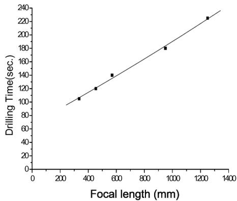
**Figure 2.** Variation of the time of drilling vs. the focal length of the lens.
