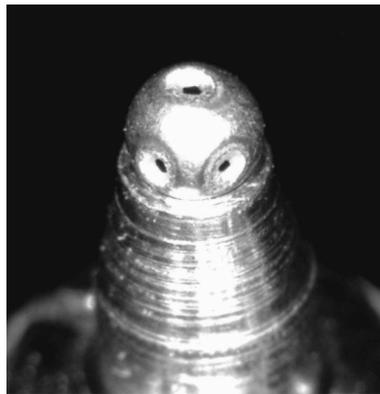
**Figure 5.** Hohlräum cavity with three holes.
