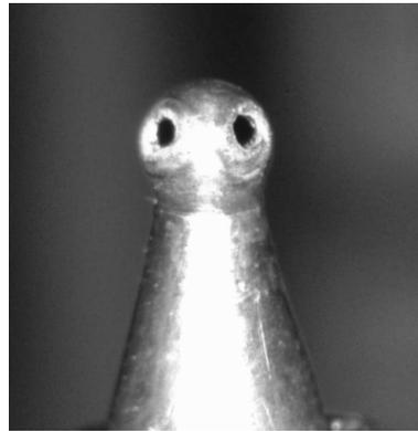
**Figure 4.** Hohlräum cavity with two holes at  $90^\circ$ .
