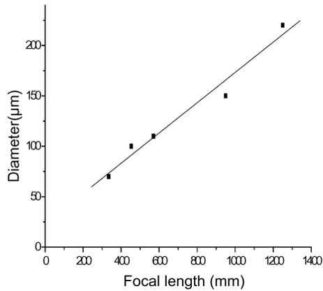
**Figure 1.** Variation of the hole diameter vs. the focal length of the lens used.
