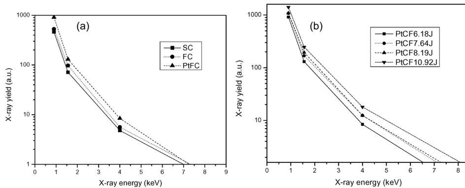
**Figure 2.** (a) X-ray spectrum recorded with various diodes covered with different X-ray filters for solid carbon (■), carbon foam (●) and Pt-doped carbon foam (▲). (b) X-ray spectrum of Pt-doped carbon foam for various laser energies.
