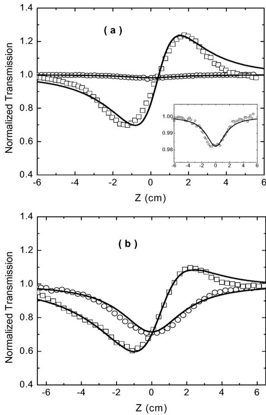
**Figure 2.** Closed- and open-aperture Z-scan profiles for (a) GG 420 and (b) OG 515 at peak intensities of  $175 \text{ GW/cm}^2$  and  $400 \text{ GW/cm}^2$ , respectively. Squares and circles are experimental closed- and open-aperture Z-scan data points, respectively and solid lines are numerically fitted curves.
