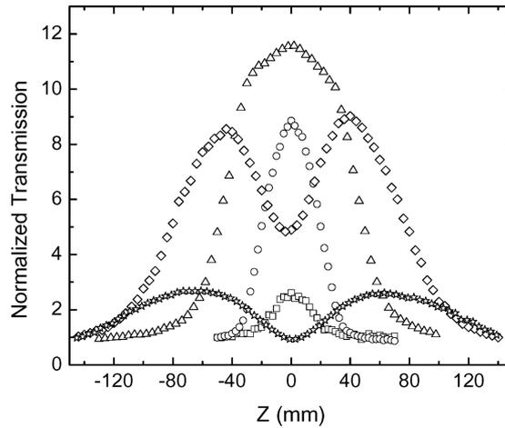
**Figure 3.** Open-aperture Z-scan profiles for RG 850 performed at intensities of 14 (squares), 50 (circles), 290 (triangles), 650 (diamonds) and  $2.5 \times 10^3$  (stars)  $\text{GW}/\text{cm}^2$ .
