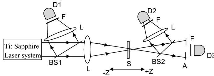
**Figure 1.** Experimental Z-scan set-up. L – lens, F – neutral density filters, BS – beam splitter, A – aperture, D – photodiode, S – sample and Z – position.
