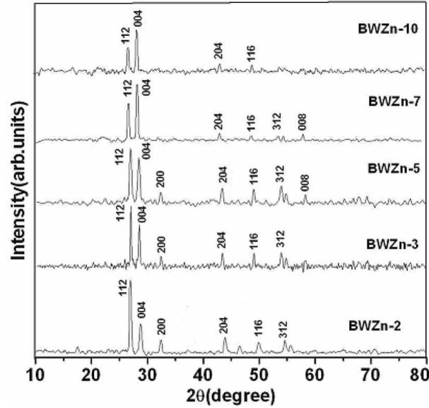
**Figure 1.** XRD pattern of ZnO-doped  $\text{WO}_4$  films post-annealed at  $T_{\text{ANN}} = 900^\circ\text{C}$ .
