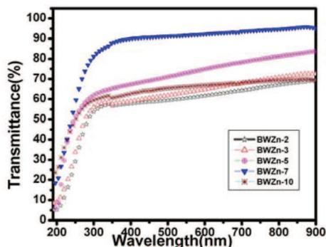
Figure 3. Transmittance spectra of the as-deposited BWZn films.
