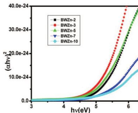
Figure 4. Tauc plots for the as-deposited BWZn films.
