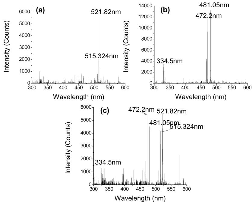
**Figure 5.** LIBS spectra of (a) copper, (b) zinc and (c) brass samples.
