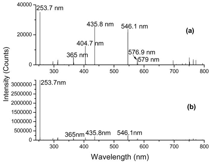
**Figure 2.** (a) Wavelength and (b) intensity calibration of the LIBS system using NIST lamps.
