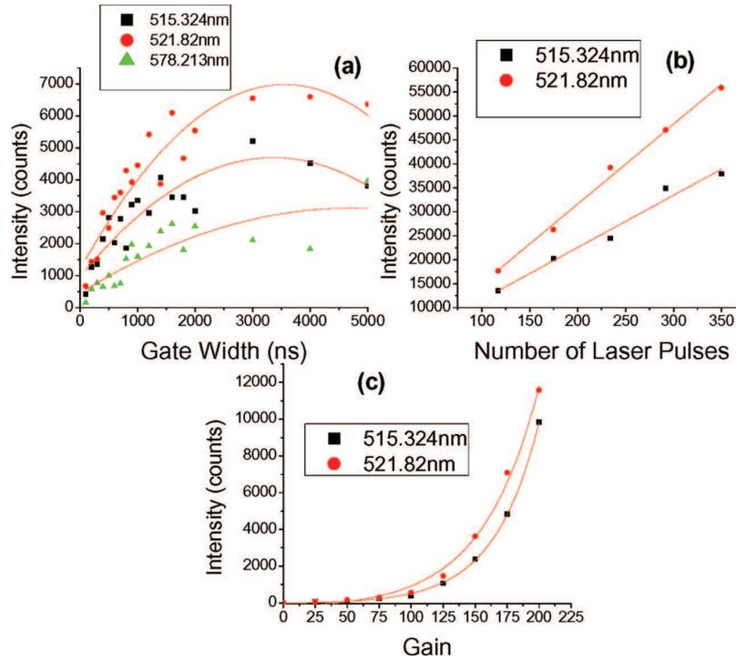
**Figure 4.** Variation in LIBS signal with (a) gate width, (b) number of laser pulses and (c) gain.
