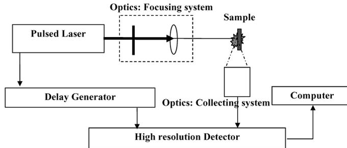
**Figure 1.** LIBS experimental set-up for multi-elemental analysis.
