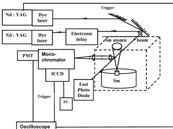
**Figure 1.** Experimental set-up for spectrally resolved two-colour laser-induced fluorescence.
