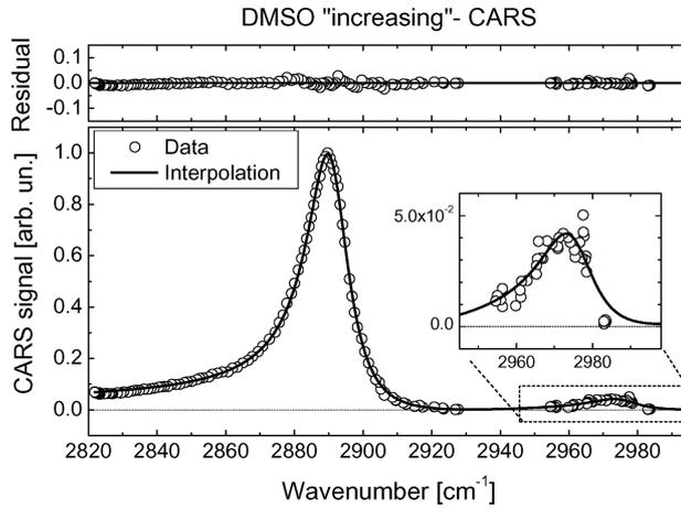
**Figure 3.** CARS signal as a function of the frequency detuning between pump and Stokes for DMSO solution.
