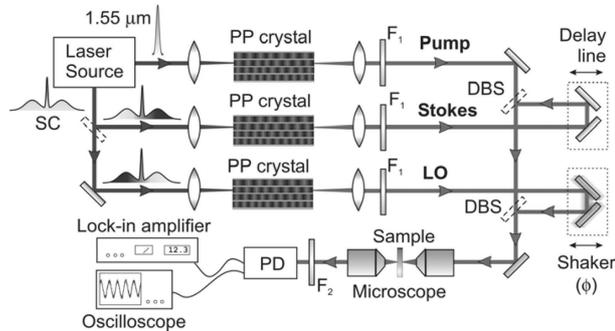
**Figure 1.** Experimental set-up. DBS: dichroic beam splitter; F1: band-pass filter; F2: short/band-pass filters; PP: periodically-poled crystals; SC: supercontinuum; PD: photodetector.
