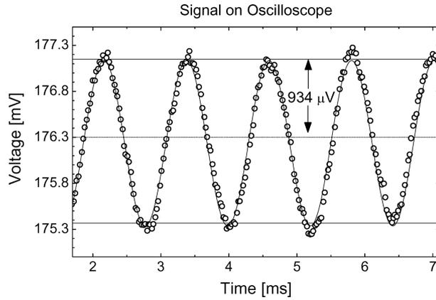
**Figure 5.** Interference pattern between CARS and LO as a function of their delay.
