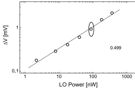
**Figure 6.** Modulation amplitude ( $\Delta V$ ) as a function of LO power.
