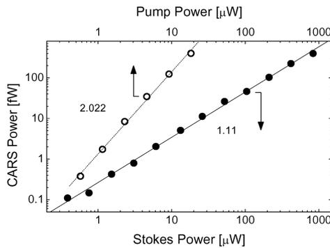
**Figure 4.** CARS power at the peak of the DMSO response as a function of pump and Stokes powers.
