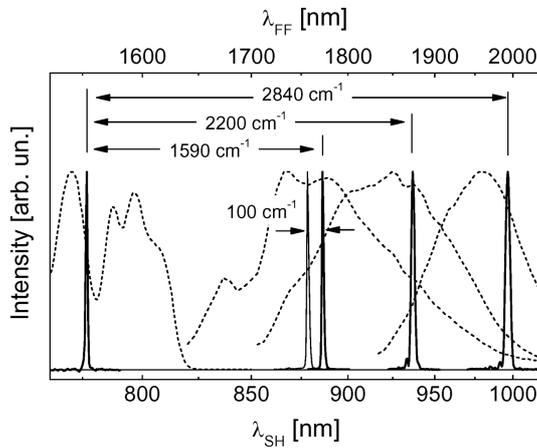
**Figure 2.** Compressed SH spectra (solid lines, bottom scale) and the corresponding FF spectra (dashed lines, top scale).
