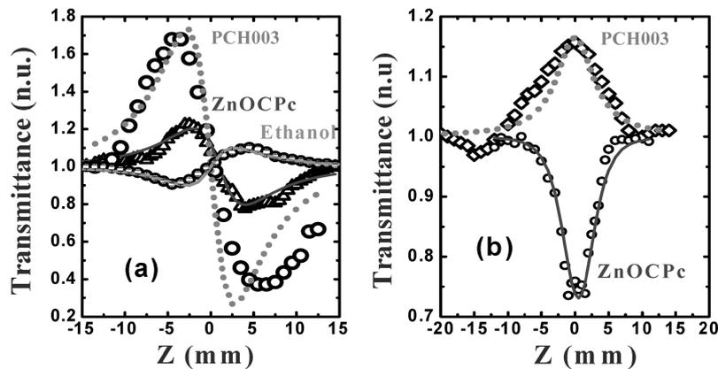
**Figure 2.** (a) Closed- and (b) open-aperture Z-scan data for ZnOCPc (in water) and PCH003 (ethanol). Ethanol (solvent) did contribute to the  $n_2$  but not to the nonlinear absorption. The lines (solid for ZnOCPc and dotted for PCH003) are fits to the experimental data. The sign of  $n_2$  was opposite compared to that of the sample.
