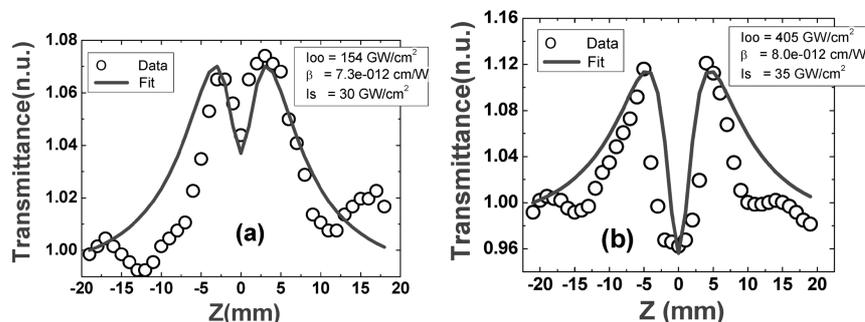
**Figure 3.** Open-aperture data of (a) PCH001 at a peak intensity of 154 GW/cm<sup>2</sup> and (b) PCH003 at a peak intensity of 405 GW/cm<sup>2</sup>. Solid lines are fits to the experimental data (open circles).
