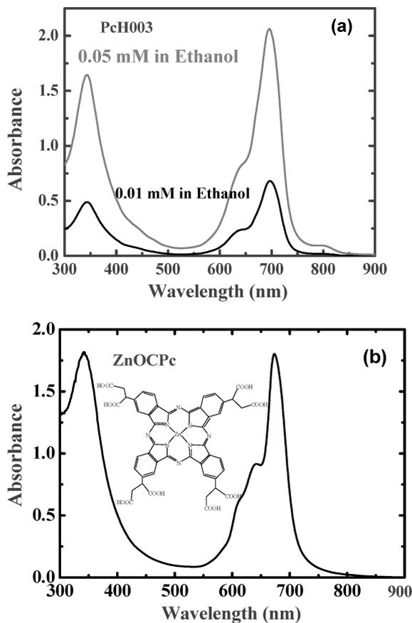
**Figure 1.** Absorption spectra of (a) PCH003 dissolved in ethanol and (b) ZnOCPc dissolved in water. Inset shows the structure.
