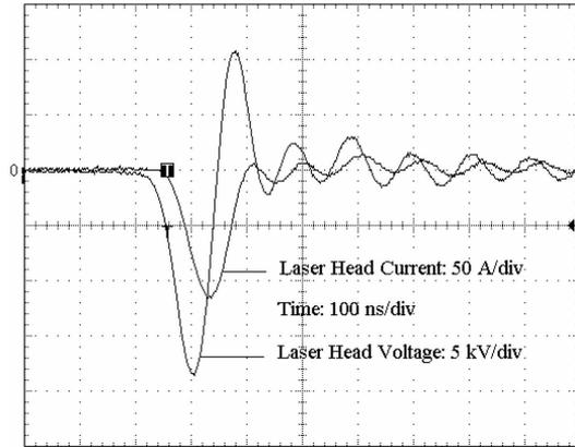
Figure 5. Laser head voltage and current waveforms.
