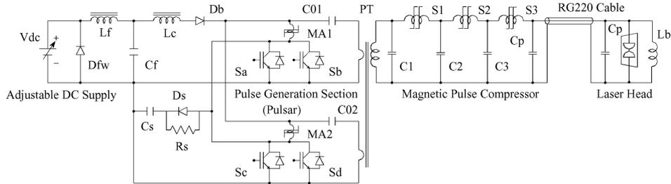
**Figure 1.** Circuit diagram of the solid-state pulsed power supply.
