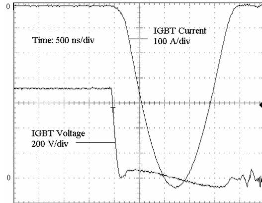
Figure 3. IGBT voltage and current waveforms.
