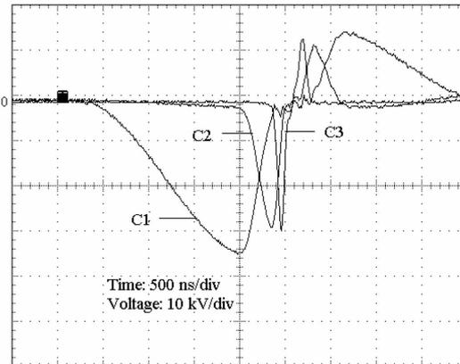
Figure 4. MPC stage voltage waveforms.
