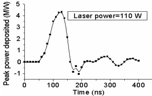
**Figure 6.** Temporal variation of the peak-deposited power in the laser tube at 110 W output power.
