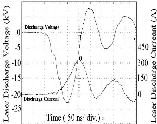
**Figure 5.** Temporal behaviour of the laser head voltage and current at 110 W laser power condition.
