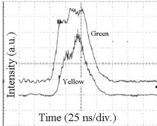
**Figure 4.** Temporal profile of green and yellow components of the copper HyBrID laser.
