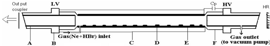
**Figure 1.** Schematic lay-out of the copper HyBrID laser. LV – low voltage side, HV – high voltage side, A – press-fitted Cu electrode, B – water-cooled SS flange, C – aluminium strips for current return, D – high purity Cu pieces, E – alumina fibre insulation, F – flared end fused silica discharge tube, Cp – peaking capacitor and HR – high reflector ( $R > 99.9\%$ ).
