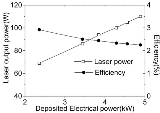
**Figure 3.** Variation of laser power and tube efficiency with deposited electrical power.
