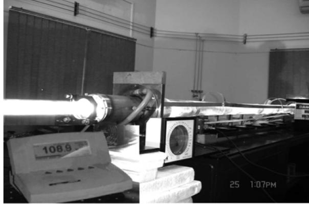
**Figure 2.** A 110 W copper HyBrID laser in operation.
