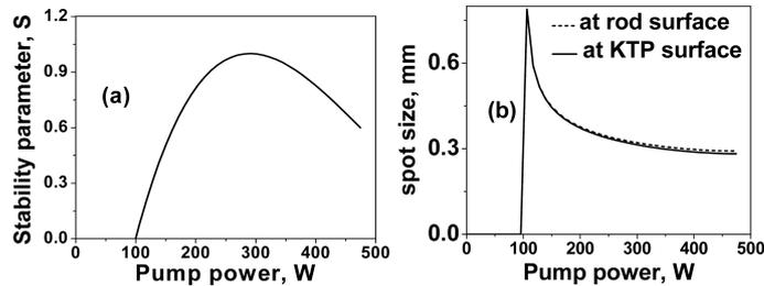
**Figure 2.** Calculated variation of the (a) stability and (b) spot sizes as a function of the pump power.
