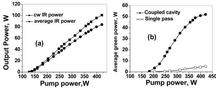
Figure 3. Measured slope efficiency curves (a) at 1064 nm and (b) at 532 nm.
