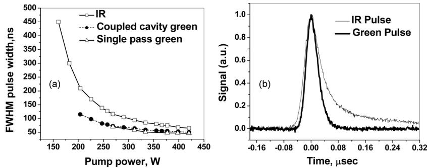
Figure 4. (a) Measured variation of pulse width with the pump power and (b) Q-switched pulse shape.
