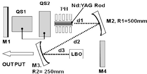
Figure 1. Schematic of experimental arrangement.
