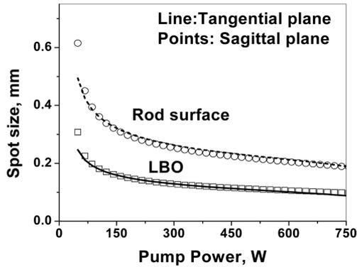
Figure 3. Calculated variation of fundamental mode size.
