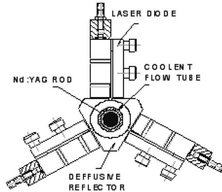
**Figure 2.** Schematic of the pump head assembly.
