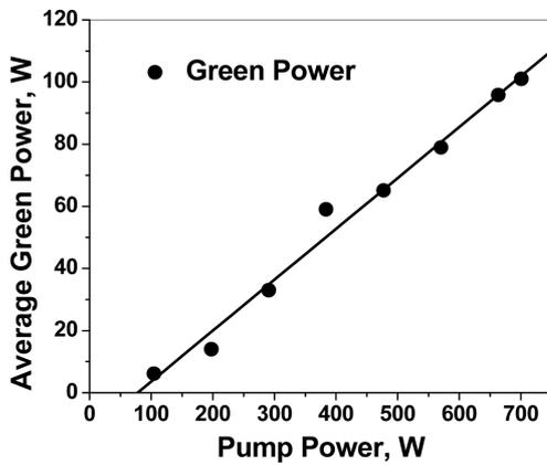
Figure 4. Green power vs. the pump power.
