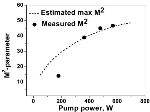
Figure 6. Calculated and measured  $M^2$  parameters.
